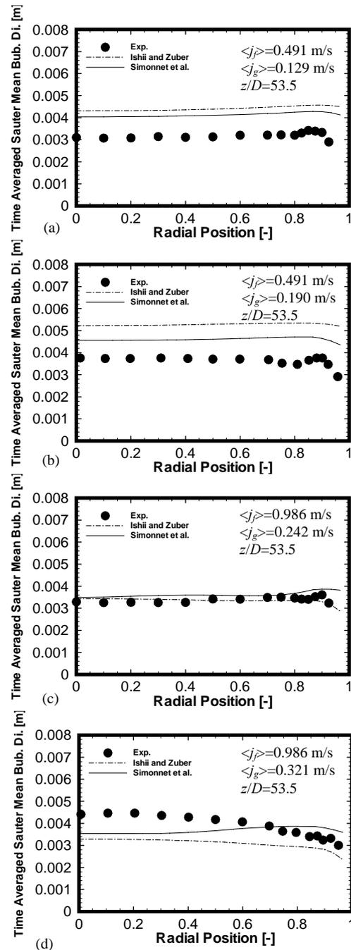
**Figure 4:** Predicted Sauter mean bubble diameter distribution and experiment data of Hibiki et al. (2001).
