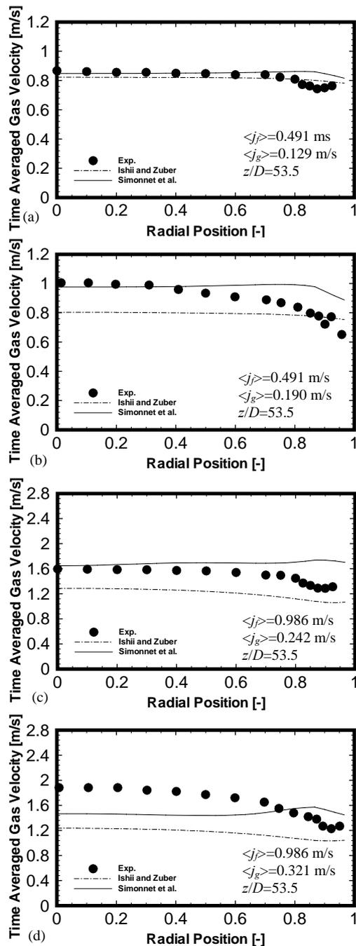
**Figure 5:** Predicted radial gas velocity profile and experiment data of Hibiki et al. (2001).
