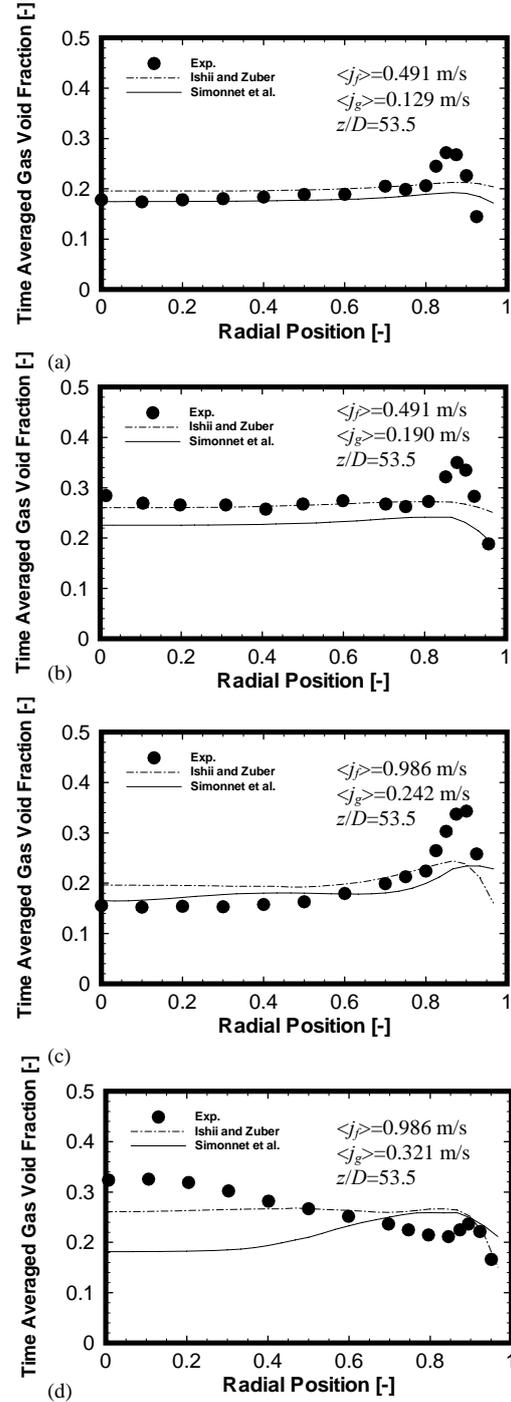
**Figure 3:** Predicted radial void fraction distribution and experiment data of Hibiki et al. (2001).
