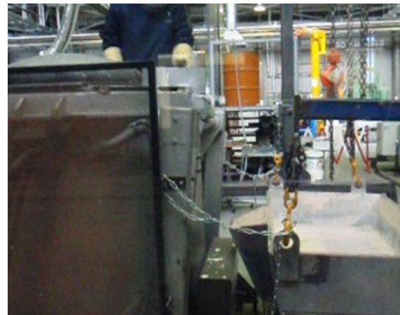
Figure 3: 500 kg tilting furnace and slung sow used for crucible pouring experiments.
