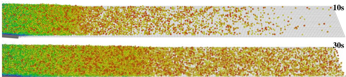
**Figure 5:** Flow over the screen for feed rate 0.250 kg/s at  $t = 10$  s (top) and 30 s (bottom). The particles are coloured by size, with blue being the smallest and red being the largest.
