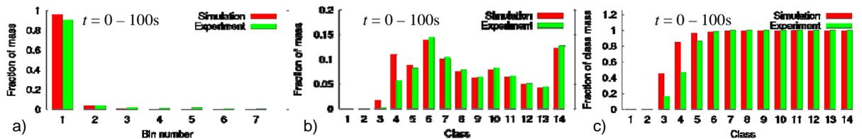
**Figure 7:** Comparisons between simulation and experiment for the 0.05 kg/s case over the full simulation time  $t = 0 - 100$  s. The figures show a) the fractions of the total collected mass contained in each bin under the screen, b) the fractions of the total collected mass that is captured in the first collection bin in each class, and c) the fraction of each class's mass that is captured in the first collection bin.
