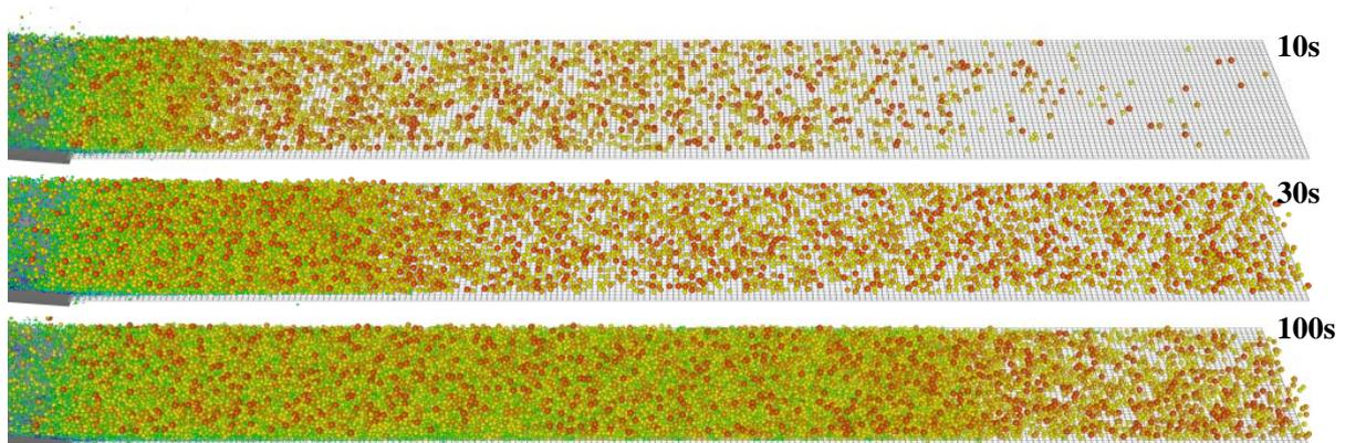
**Figure 3:** Flow over the screen for feed rate 0.125 kg/s at  $t = 10$  s (top), 30 s (middle) and 100 s (bottom). The particles are coloured by size, with blue being the smallest and red being the largest.
