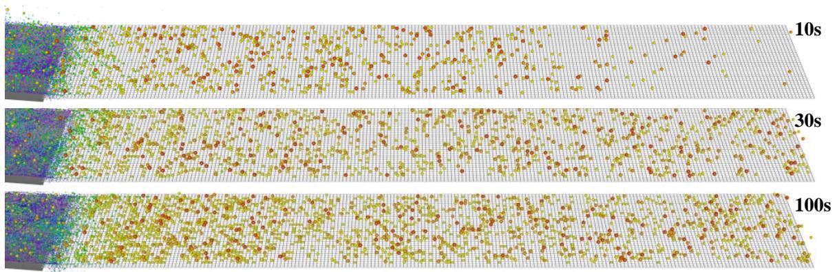
**Figure 2:** Flow over the screen for feed rate 0.05 kg/s at  $t = 10$  s (top), 30 s (middle) and 100 s (bottom). The particles are coloured by size, with blue being the smallest and red being the largest. The system very quickly stabilizes with material smaller than the screen aperture size rapidly falling through the cloth near the start of the screen.
