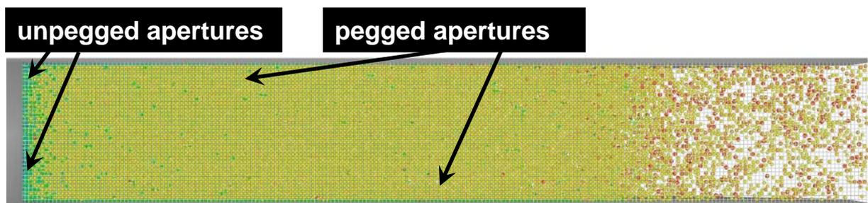
**Figure 4:** Underside of the screen for the mid feed rate of 0.125 kg/s at  $t = 100$  s. The apertures of the screen become pegged by the near aperture sized material (coloured yellow) blocking the holes and inhibiting screening. There is a small region at the start of the screen, just after the impact plate, where there is very little pegging.
