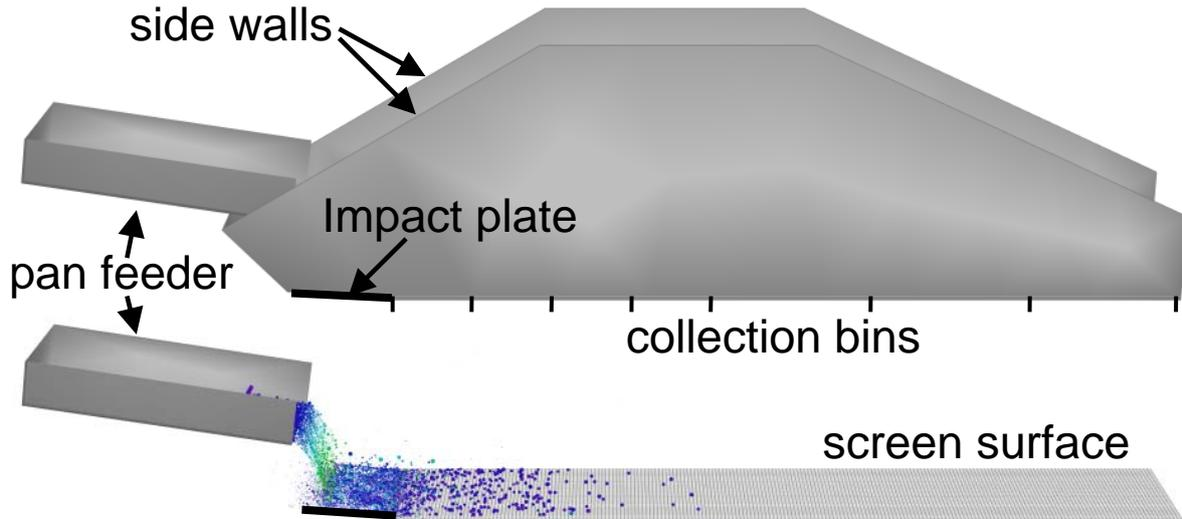
**Figure 1:** CAD model of the configuration used in the experiments and simulations. The top image shows the setup with the side walls in place. The bottom image has the side walls removed so that the screen surface is visible. A flow of particles is fed onto the impact plate from a pan feeder and then flows onto the screen surface due to its vibration.
