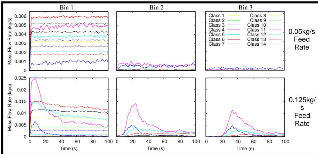
**Figure 6:** Flow rates through the first, second and third collection bins, for feed rates of 0.05 kg/s and 0.125 kg/s. The numbered classes correspond to those described in Table 2.
