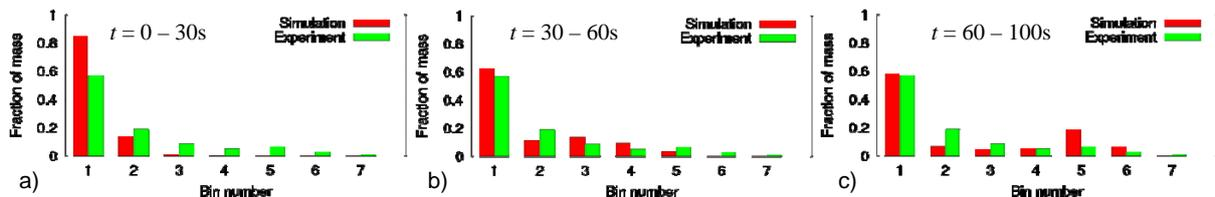
**Figure 8:** The figures show the fraction of mass captured in each collection bin under the screen during for the 0.125 kg/s feed rate, at three time frames during the simulation: a)  $t = 0-30$  s, b)  $t = 30-60$  s and c)  $t = 60-100$  s. The experimental data is also plotted on each graph for comparison.
