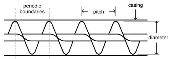
**Figure 1:** Standard pitch, single flight screw conveyor.
