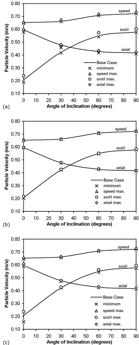
**Figure 5:** Particle velocities versus conveyor inclination: (a) for the full range of particle shapes, (b) for the full range of particle-particle frictions, and (c) for the full range of particle-boundary frictions.
