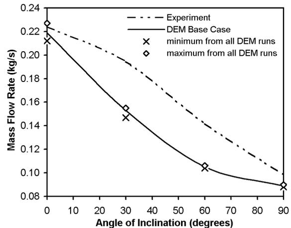
**Figure 4:** Mass flow rate versus conveyor inclination.
