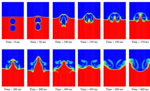
**Figure 7:** CFD model predicted behaviour of two 80-mm gas bubbles in an aqueous glycerol bath.
