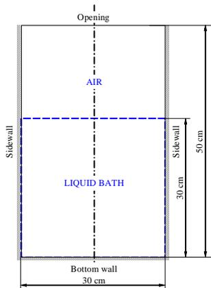
**Figure 3:** Two-dimensional computation domain defined in the CFD model (cf., Figures 1 and 2).
