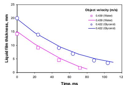
**Figure 11:** Measured and predicted variations of liquid film thickness with time in aqueous glycerol and water baths. (Symbols stand for physical model measurements and curves for CFD model predictions.)
