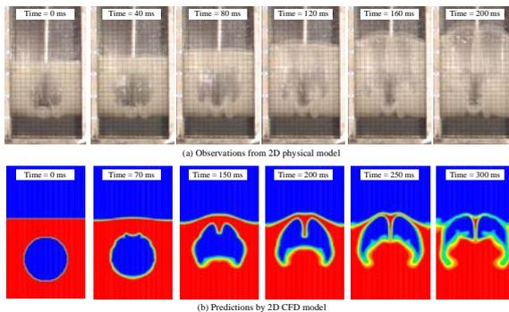
**Figure 6:** CFD model predicted behaviour of a 160-mm gas bubble in an aqueous glycerol bath in comparison with observations from the physical model (cf., Figure 1).
