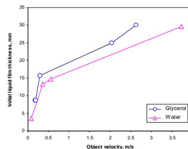
**Figure 10:** Measured liquid film thicknesses in aqueous glycerol and water baths in physical model for different object rising velocities.
