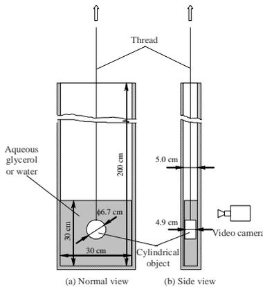
**Figure 2:** Schematic diagram of two-dimensional physical model set-up for liquid film thickness measurement.
