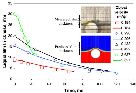
**Figure 5:** Comparison between variations of the liquid film thickness measured on the solid object top surface in the physical model (cf., Figure 2) for different object rising velocities and those predicted by the CFD model. (Symbols stand for physical model measurements and curves for CFD model predictions.)
