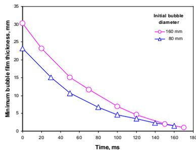
**Figure 9:** CFD model predicted variations in minimum film thickness of two different size gas bubbles in aqueous glycerol bath with time.
