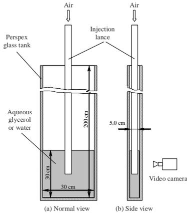
**Figure 1:** Schematic diagram of a two-dimensional physical model set-up of the CSIRO pilot plant furnace.
