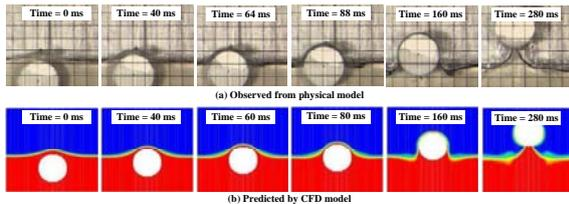
**Figure 4:** Comparison between the motion of a cylindrical object rising out of an aqueous glycerol bath in the physical model (cf., Figure 2) and that simulated by the CFD Model (object rising velocity = 0.296 m/s).
