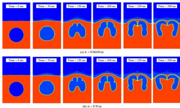
**Figure 12:** Comparison between the ANSYS CFX simulation results on the motion of a 160-mm gas bubble in an aqueous glycerol bath in the physical model (shown in Figure 1) with and without considering the surface tension effect.
