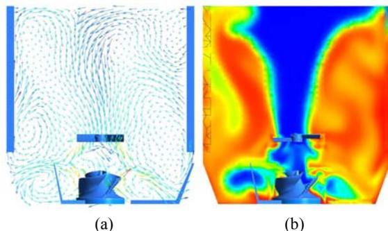
**Figure 5:** CFD results for the Case II (a) Normalised velocity vector plot (b) Liquid volume fraction profile (Legends are same as in the Figure 4)
