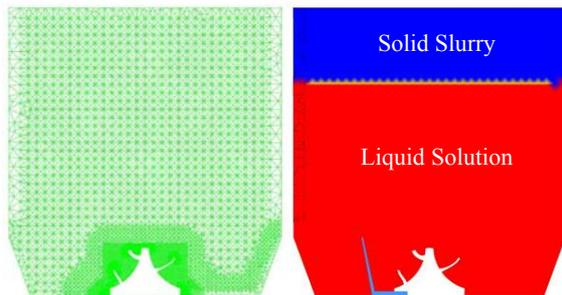
**Figure 1:** (a) Mesh generated for Case I (b) Initial volume fraction profile of Liquid solution for Case I.
