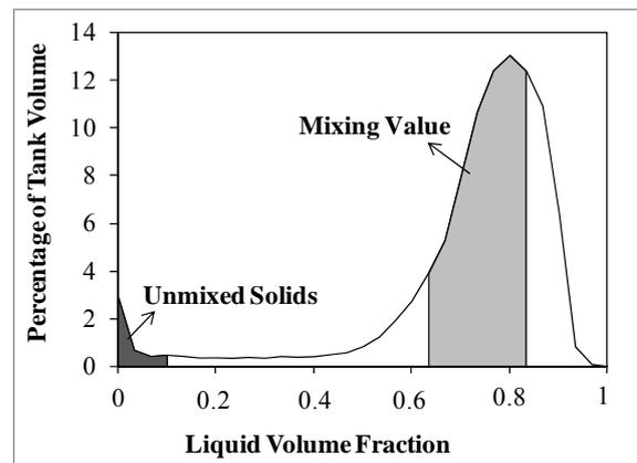
**Figure 2:** Typical liquid volume fraction values across the tank volume
