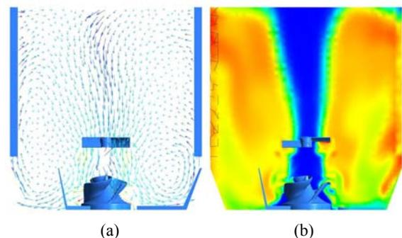
**Figure 6:** CFD results for the Case III (a) Normalised velocity vector plot (b) Liquid volume fraction profile (Legends are same as in the Figure 4)
