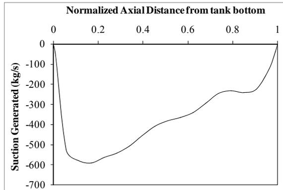
**Figure 3:** Typical variation of suction created with the normalised axial distance from the tank bottom
