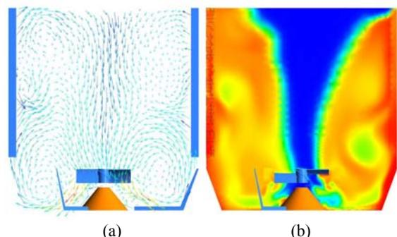
**Figure 9:** CFD results for the Case VI (a) Normalised velocity vector plot (b) Liquid volume fraction profile (Legends are same as in the Figure 4)
