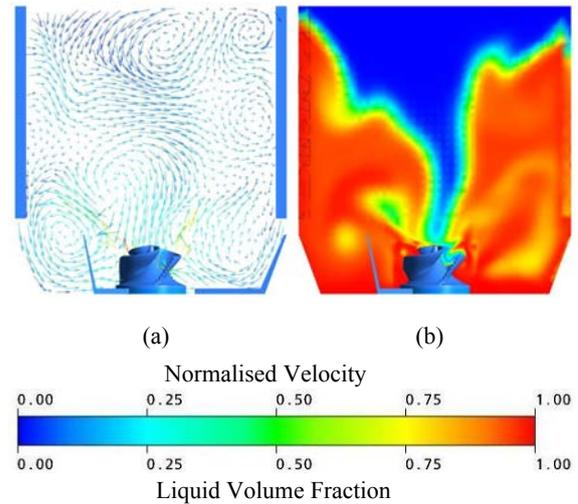
**Figure 4:** CFD results for the Case I (a) Normalised velocity vector plot (b) Liquid volume fraction profile
