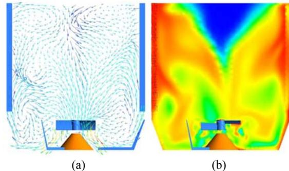
**Figure 8:** CFD results for the Case V (a) Normalised velocity vector plot (b) Liquid volume fraction profile (Legends are same as in the Figure 4)
