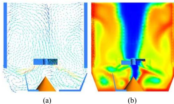
**Figure 7:** CFD results for the Case IV (a) Normalised velocity vector plot (b) Liquid volume fraction profile (Legends are same as in the Figure 4)
