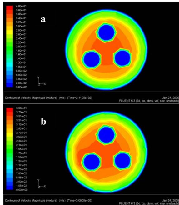
**Figure 11:** Gas velocity pattern on the furnace top (a) during normal tapping and (b) during the taphole gassing situation
