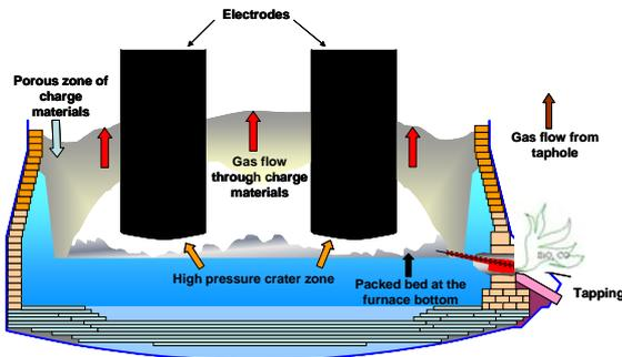
**Figure 1:** Schematic of submerged arc furnace used for Silicon production.
