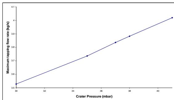
**Figure 7:** Maximum tapping flow rate increases with increase of crater pressure.
