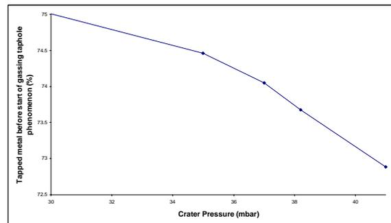
**Figure 9:** Percentage of total metal in the furnace before gassing taphole phenomenon starts.
