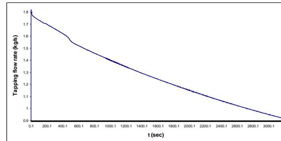
**Figure 4:** Tapping flow rate of silicon melt from the furnace taphole without excess gas pressure.
