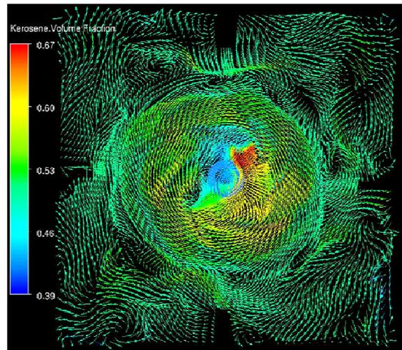
**Figure 9C** LES based Instantaneous Flow structures in Multiphase Operation at Impeller at XY Plane  $z=0.185$  location.
