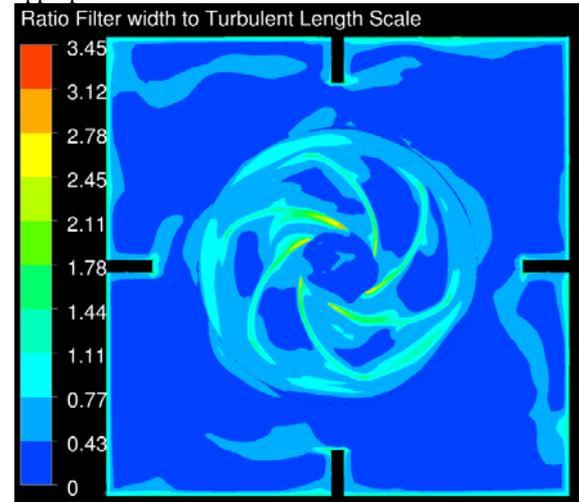
**Figure 2:** A contour of ratio of Grid length to Turbulent length that measures sufficiency of grid size.
