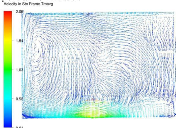
Figure 6B. Smagorinsky LES predicted time averaged profile at  $x=-0.112$  location.
