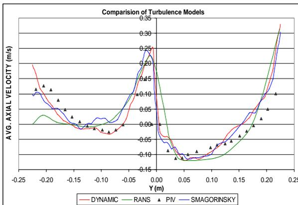
**Figure 7:** Comparison of Turbulence Models
