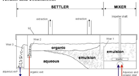
Figure 1: Schematic diagram of geometry.
