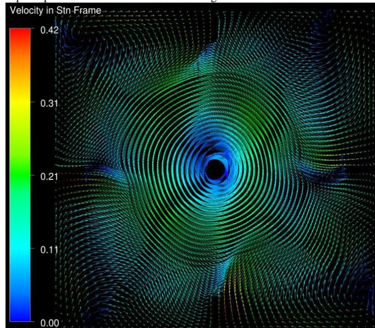
**8A.** RANS Model Prediction of Mean Velocity at XY Plane at  $z=0.42$  height.
