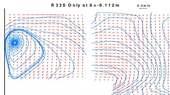
Figure 6A. PIV Experimental Snapshot of time averaged profile at  $x=-0.112$  location.
