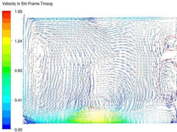
**Figure 6C.** Dynamic LES predicted time averaged profile at  $x=-0.112$  location.
