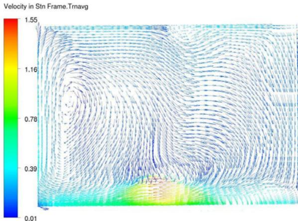
**Figure 6D.** RANS Model predicted time averaged profile at  $x=-0.112$  location.
