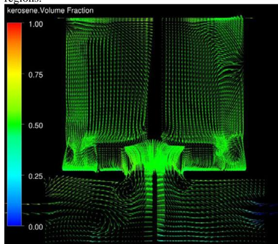
**Figure 9A** RANS Model Prediction of Mean Velocity and Dispersion in Multiphase system at  $x=0$  location.
