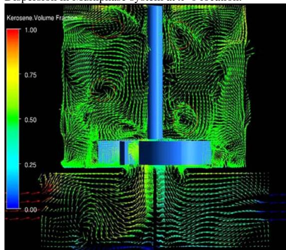
**Figure 9B** LES based Instantaneous Flow structures and dispersion in Multiphase operation at  $x=0$  location.
