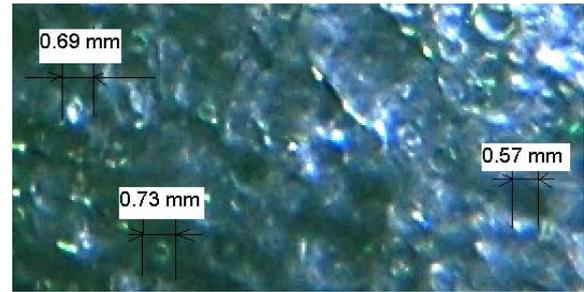
Figure 5: Droplet size measurements in the mixer – geometrical centre of the mixer wall.
