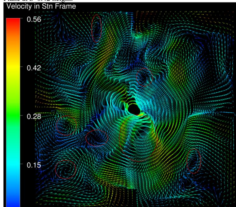
**8B.** LES prediction of Instantaneous Flow at XY Plane at  $z=0.42$  height.
