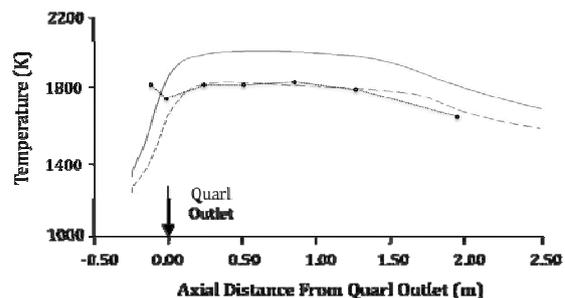
**Figure 1:** Centre line temperature profile of the IFRF furnace for; experimental results (o), single injection with a Rosin-Rammler size distribution (—), and multiple injections with a uniform size distribution (---).
