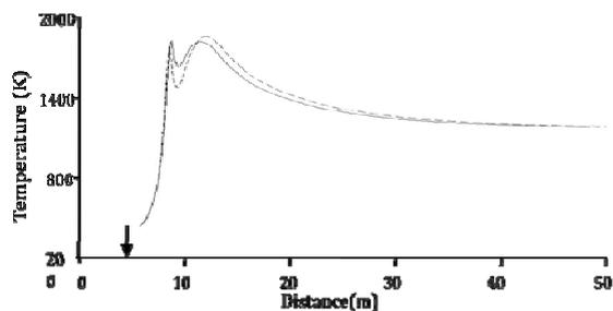
**Figure 5:** Centre line temperature profile of the McDonalds Lime kiln for a coal flow rate of 0.7594 kg/s (—) and 0.8594 kg/s (---).
