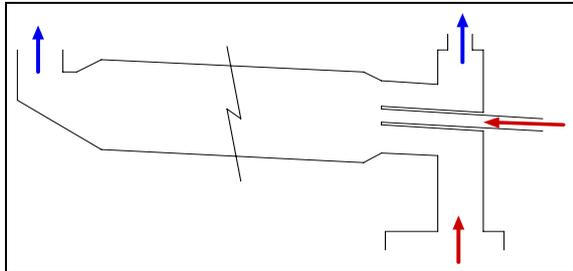
**Figure 3:** Schematic showing inlets (red) and outlets (blue) of the McDonald's Lime kiln model.
