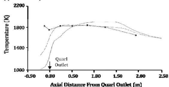
**Figure 2:** Centre line temperature profile of the IFRF furnace for; experimental results (o), mixture fraction/PDF approach (—), and finite rate approach (---).
