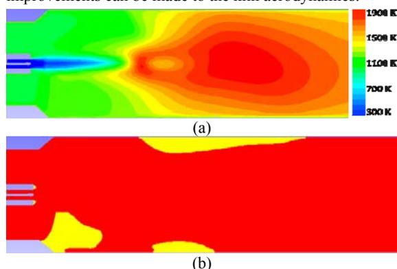
**Figure 4:** (a) Temperature profile in the flame region of the McDonalds Lime kiln (b) Contours of positive (red) and negative (yellow) z-direction velocity.
