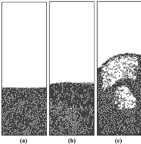
**Figure 9:** Solid configurations at dynamically stable state when the density of jetsam particles is 2500 kg m<sup>-3</sup> and the density of flotsam particles is 4000 kg m<sup>-3</sup> at gas injection velocities: (a) 0.7 m s<sup>-1</sup>, (b) 0.8 m s<sup>-1</sup>, (c) 1.25 m s<sup>-1</sup>.
