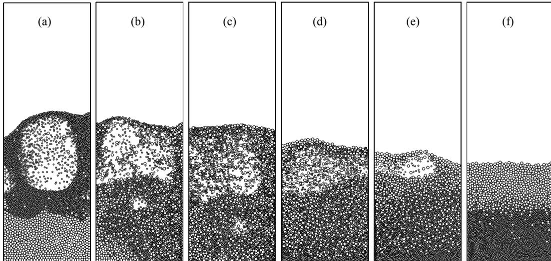
**Figure 3:** Solid configurations at dynamically stable states showing the transition from normal segregation to inverse segregation at the gas injection velocity  $1.0 \text{ m s}^{-1}$  when the density of flotsam particles is: (a) 2500, (b) 3000, (c) 4000, (d) 5000, (e) 6000, (f) 6500  $\text{kg m}^{-3}$ .
