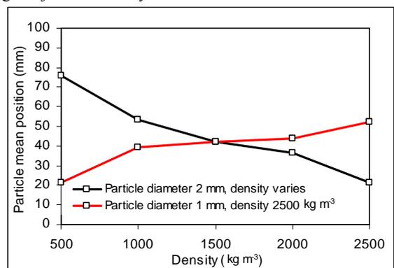
**Figure 8:** Vertical mean position of each type particles at dynamically stable state at different densities of large size particles when the gas injection velocity is  $0.8 \text{ m s}^{-1}$ .
