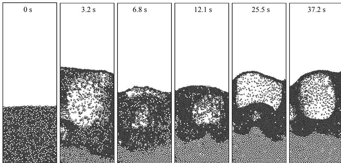
**Figure 1:** Solid configuration at different times showing normal segregation process with flotsam particles residing on the top of jetsam particles when the gas injection velocity is  $1.0 \text{ m s}^{-1}$  and the densities of both flotsam and jetsam particles are  $2500 \text{ kg m}^{-3}$  (Feng and Yu, 2007).
