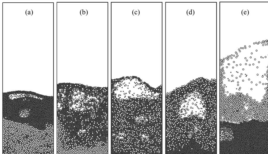
**Figure 4:** Solid configurations at dynamically stable states showing the transition from normal segregation to inverse segregation at the gas injection velocity  $0.8 \text{ m s}^{-1}$  when the density of jetsam particles is: (a) 2500, (b) 2000, (c) 1500, (d) 1000, (e) 500  $\text{kg m}^{-3}$ .
