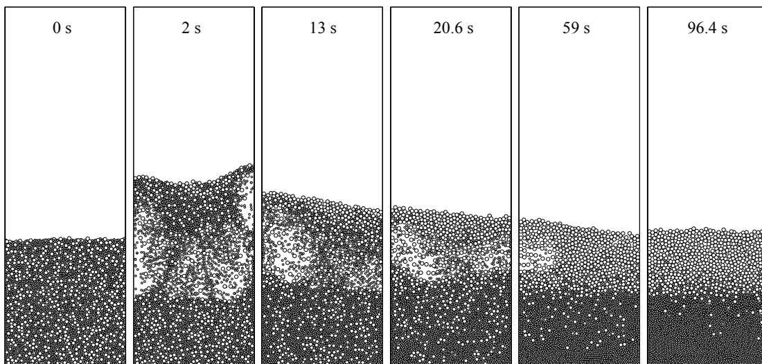
**Figure 2:** Solid configuration at different times showing inverse segregation process with jetsam particles residing on the top of flotsam particles when the gas injection velocity is  $1.0 \text{ m s}^{-1}$  and the densities of flotsam and jetsam particles are respectively  $6500$  and  $2500 \text{ kg m}^{-3}$ .
