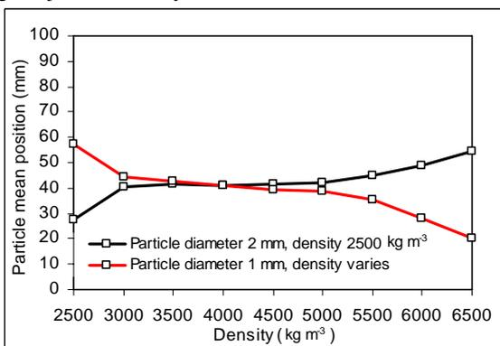
**Figure 6:** Vertical mean position of each type particles at dynamically stable state at different densities of small size particles when the gas injection velocity is  $1.0 \text{ m s}^{-1}$ .
