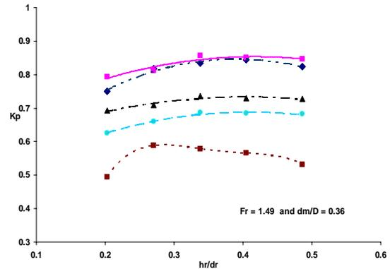
**Figure 2:** The Influence of the draft tube distance on pumping efficiency for: (♦) homogeneous solution (■) monodisperse suspension  $l=0.35\text{mm}$ ,  $\Delta\rho=525(\text{kg}/\text{m}^3)$  (▲) monodisperse suspension  $l=0.35\text{mm}$ ,  $\Delta\rho=700(\text{kg}/\text{m}^3)$
