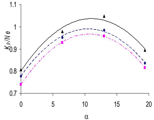
**Figure 6:** The Influence of the draft tube opening angle  $\alpha$  on the hydraulic efficiency of the apparatus for: (×) monodisperse alum suspension  $l=0.5\text{mm}$ ,  $\Delta\rho=700(\text{kg/m}^3)$ , (▲) monodisperse alum suspension  $l=0.35\text{mm}$ ,  $\Delta\rho=700(\text{kg/m}^3)$  (■) monodisperse ammonia sulphate suspension  $\Delta\rho=500(\text{kg/m}^3)$ .
