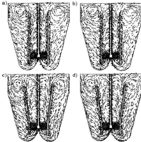
**Figure 7:** Fluid flow profiles: a,c –mother liquid, b,d – polydisperse suspension
