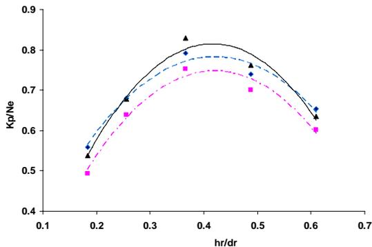
**Figure 3:** The Influence of the draft tube distance on the hydraulic efficiency of the apparatus for: (x) monodisperse alum suspension  $l=0.5\text{mm}$ ,  $\Delta\rho=700(\text{kg/m}^3)$ , (▲) monodisperse alum suspension  $l=0.35\text{mm}$ ,  $\Delta\rho=700(\text{kg/m}^3)$  (■) monodisperse ammonia sulfate suspension
