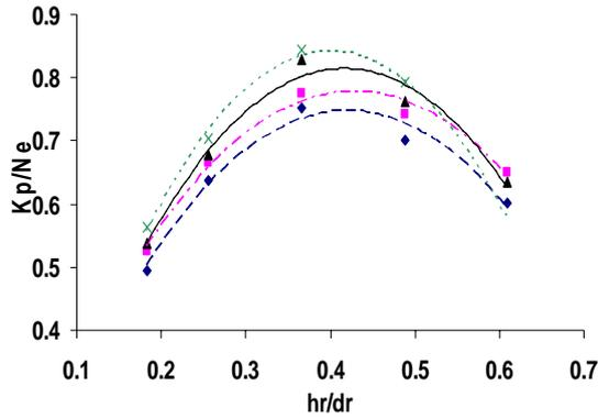
**Figure 4:** The Influence of the draft tube distance on hydraulic efficiency of the apparatus for: (■) monodisperse suspension  $l=0.35\text{mm}$ ,  $\Delta\rho=700(\text{kg/m}^3)$ , (◆) monodisperse suspension  $l=0.35\text{mm}$ ,  $\Delta\rho=500(\text{kg/m}^3)$ , (×) polydisperse suspension,  $\Delta\rho=700(\text{kg/m}^3)$ , (▲) polydisperse  $=500(\text{kg/m}^3)$ .
