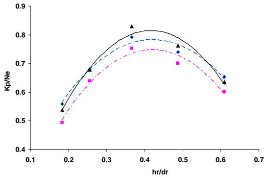
**Figure 3** shows the influence of the draft tube distance on hydraulic efficiency of the apparatus for the flow of monodisperse suspensions of ammonium sulphate and alum for two particle sizes: 0.35mm and 0.5mm. It can be noticed that the area of the best hydraulic efficiency is for the draft tube distance within the range of 0.35 and 0.5  $h_r/d_r$ . Higher hydraulic efficiency for alum is caused by the lower suspension density. The power number is inversely proportional to the density.
