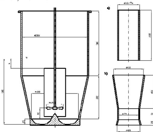
**Figure 1:** Conical-Cylindrical mixing unit.
