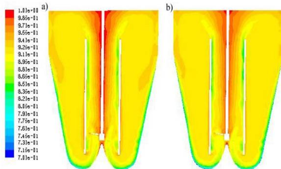
**Figure 5:** Bed porosity distribution in DTM apparatus of the draft tube distance of  $h_r/d_r=0.36$ ,  $\Delta\rho =500(\text{kg/m}^3)$  monodisperse suspension  $l=0.35\text{mm}$ , b) polydisperse suspension
