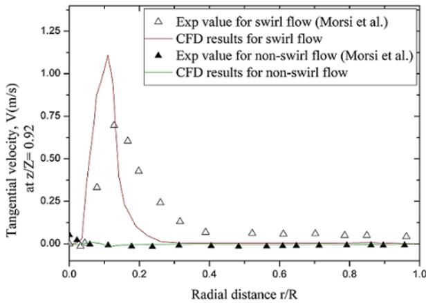
**Figure 1(c):** Mean tangential velocity comparison between swirl and non-swirl flow (TSL) (Huda et al 2009).
