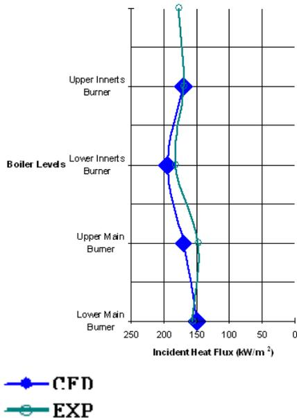
**Figure 5(d)** Comparison of measured incident heat flux on the wall with prediction (Achim et al 2009).
