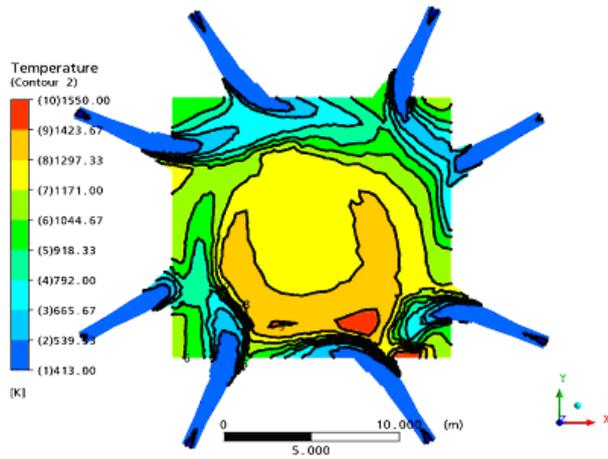
**Figure 5(c)** Temperature contours on Lower Boiler Plane (Achim et al 2009).
