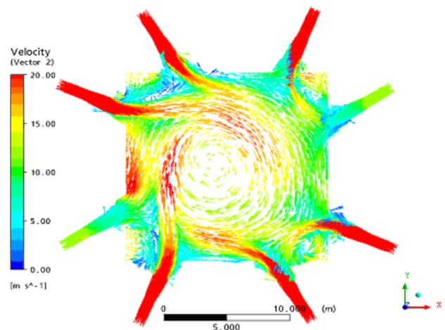
**Figure 5(b)** Velocity Vectors on Lower Boiler Plane (Achim et al 2009).
