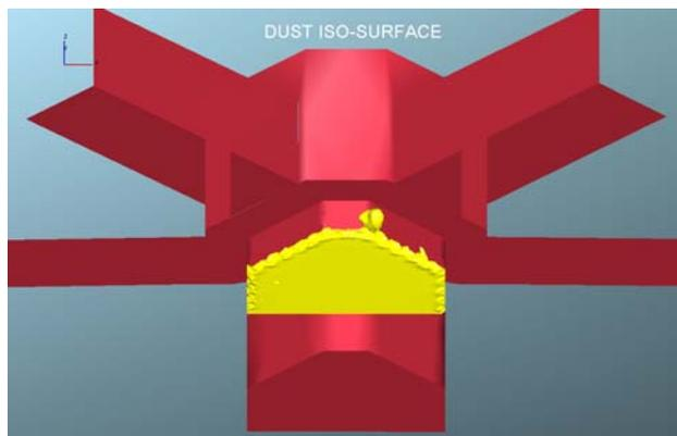
**Figure 3(c)** Dust iso-contours or iso-surface ( $100\text{mg}/\text{m}^3$ ) exit through holes (proposed system) (Naser et al. 2008).
