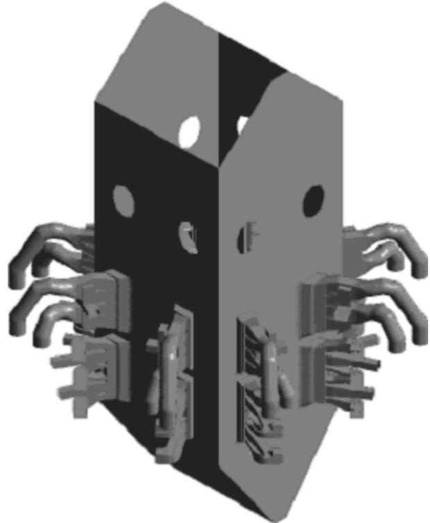
**Figure 5(a)** Full scale tangentially fired boiler with mill ducting (Achim et al 2009).
