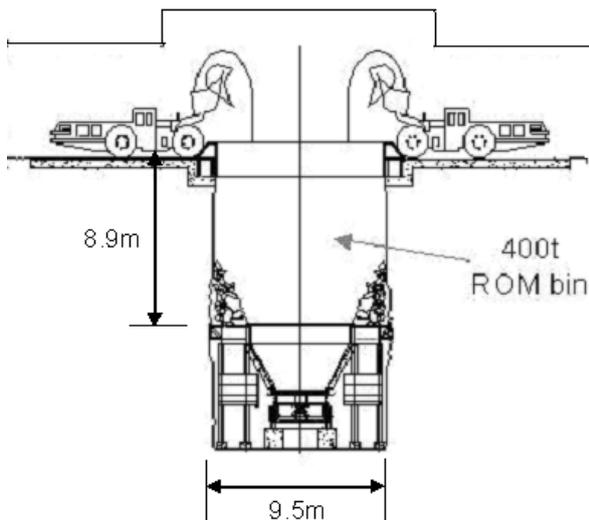
**Figure 3(a)** Typical LDH trucks tipping into a ROM bin (Naser et al. 2008).
