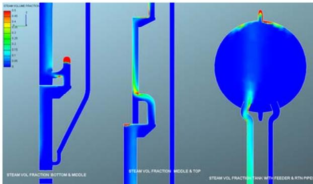
**Figure 4(c)** Steam volume fraction on a vertical plane through the middle of the jackets (showing side view). The colour key varies uniformly from 0.0 (blue) to 0.9 (red)
