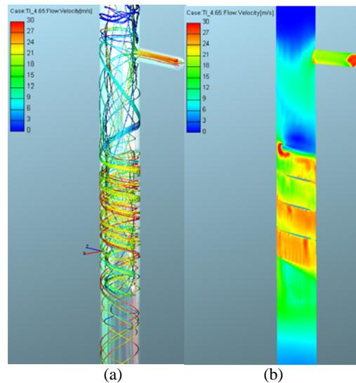
**Figure 6 (a)** Velocity streamlines showing the flow path of air and **(b)** velocity in the near wall regions (Ahmed et al. 2009)
