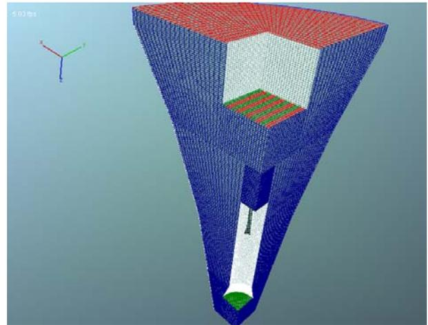
**Figure 2(a)** The computational grid used for concentrator bin.
