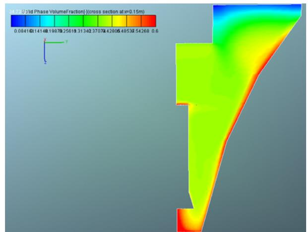
**Figure 2(b)** Solid-phase volume fraction, showing accumulation on the slanting wall. The colour key varies uniformly from 0.0 (blue) to 0.6 (red)
