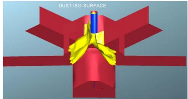
**Fig. 3(d).** Dust iso-contours or iso-surface ( $100\text{mg}/\text{m}^3$ ), exit through top of tipples (existing system) (Naser et al. 2008).
