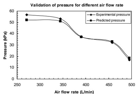
**Figure 6(c)** Validation of the predicted pressure between the inlet and air outlet for different air flow rates (Ahmed et al. 2009).
