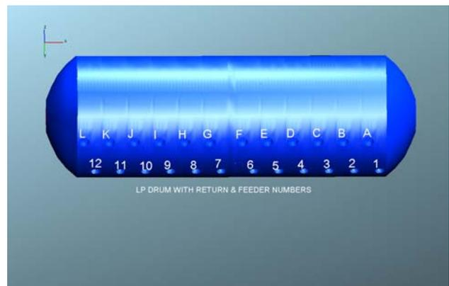
**Figure 4(a)** Geometry of LP Drum showing jacket returns & jacket feeders
