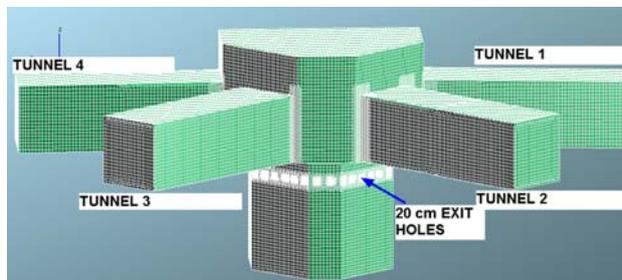
**Figure 3(b)** A typical computational grid used, exit through holes (Naser et al. 2008).
