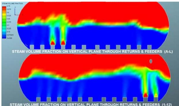
**Figure 4(d)** Steam volume fraction on a vertical plane through returns and feeders. The colour key varies uniformly from 0.0 (blue) to 0.9 (red)
