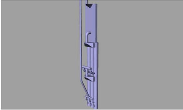
**Figure 4(b)** Geometry of typical cooling jacket set (zoomed)
