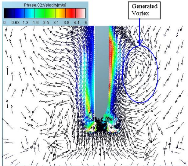
**Figure 1(b)** Velocity vectors for liquid phase (m/s) (TSL) (Huda et al 2009).
