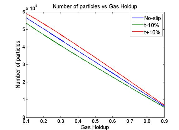
**Figure 6:** Number of SPH particles for a spatial resolution of 5mm. Note the (much smaller) volume of liquid in the tangential inlet is not included here.
