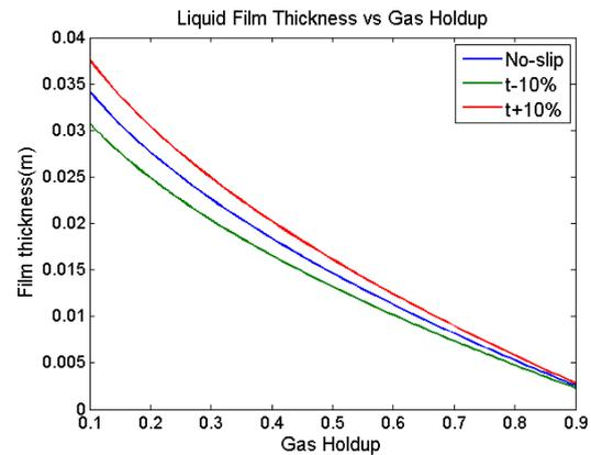
**Figure 4:** Plot of liquid film thickness versus gas holdup. The three solutions are for the no gas/liquid slip and perturbed solutions.
