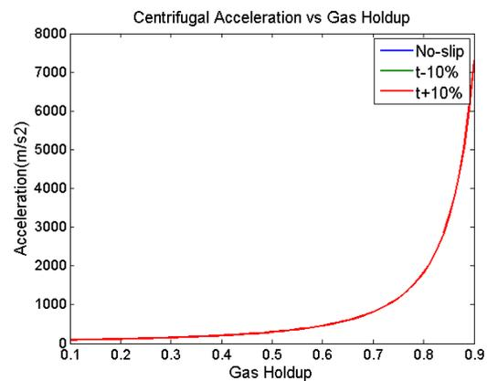
**Figure 8:** Centrifugal acceleration versus gas holdup for no slip and perturbed cases. Note that the lack of dependence on film thickness makes the three solutions identical.
