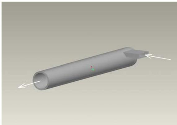
**Figure 2:** Simplified CAD model of rotating flow test case. The gas/liquid mixture enters through the tangential inlet (top right) and leaves through the pipe section (bottom left).
