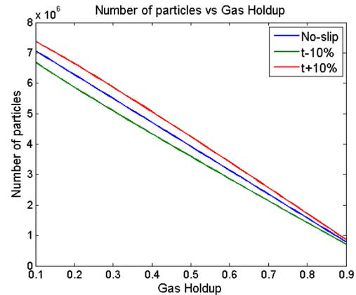
**Figure 7:** Number of SPH particles for a spatial resolution of 1mm. Note the (much smaller) volume of liquid in the tangential inlet is not included here.
