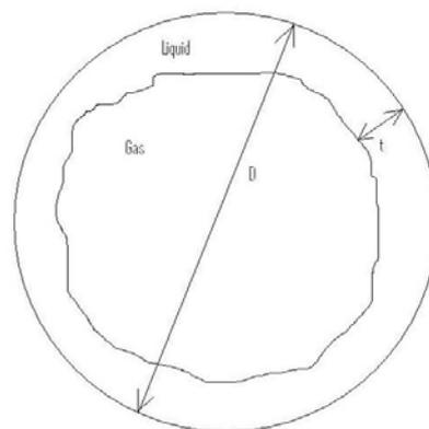
**Figure 3:** Cross section of rotating flow test case showing gas/liquid interface. This section is taken a few diameters downstream of the tangential inlet.
