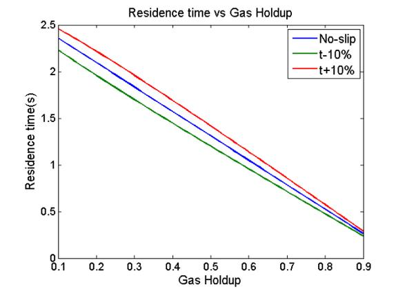
**Figure 5:** Residence time for liquid plotted versus gas holdup for no slip and perturbed cases.
