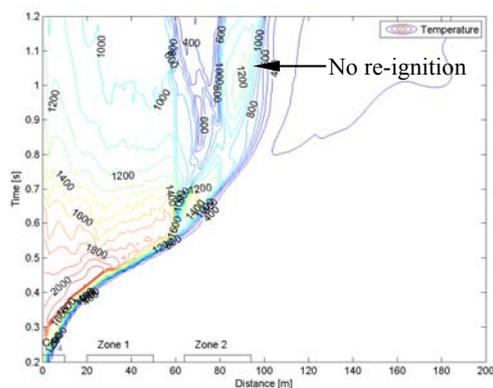
**Figure 9:** Triple ring,  $100\ \mu\text{m}$  droplets,  $200\ \text{l/s}$  flow rate
