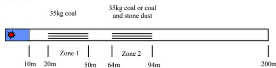
**Figure 2:** Kloppebos tunnel layout – double strong coal dust explosion (not to scale)
