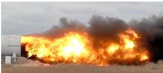
**Figure 3:** Results of a “seminar” coal dust explosion at Kloppebos
