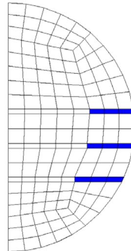
Figure 4: Tunnel mesh cross-section
