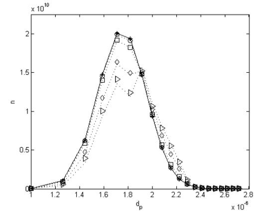
Figure 5: Change of particle size distribution over height ( $\circ$  1m,  $\square$  5m,  $\diamond$  25m and  $\triangleright$  50m) in the vertical pipe. Comparison between Smoluchowski (....) and Bus-Stop model ( $\circ$ ,  $\square$ ,  $\diamond$  and  $\triangleright$ ).
