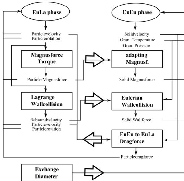
**Figure 1:** Schematic diagram of EUgran+Poly, (Schellander et al., 2012b)
