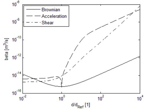
**Figure 2:** Schematic diagram, showing the agglomeration rate amount of the different effects for a  $d_{\text{Ref}} = 1 \mu\text{m}$  particle.
