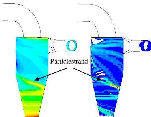
**Figure 6:** Volume fraction of granular material in the cyclone. On the left side, the Eulerian-Eulerian granular phase and on the right side the coupled Lagrangian tracer trajectories can be seen.
