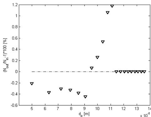
**Figure 7:** Difference of particle size distribution at the inlet and the particle outlet of the cyclone.
