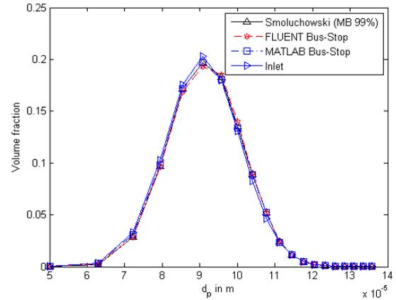
Figure 4: Comparison of particle volume fraction between discretized Smoluchowski model and the Bus-Stop model (in MATLAB and FLUENT)
