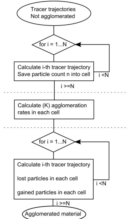
Figure 3: Schematic diagram of the Bus-Stop model.
