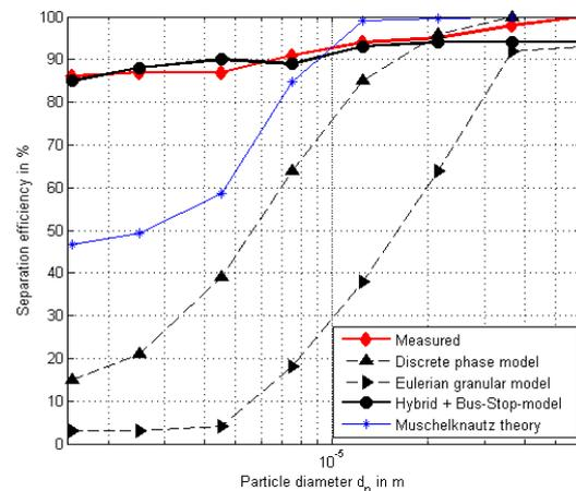
**Figure 8:** Simulation results of separation efficiency of a cyclone separating limestone granular. The results are compared to measurements and the theoretical curve computed with Muschelknautz theory.
