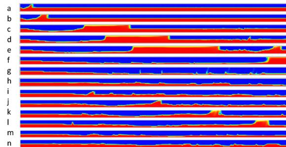
**Figure 8:** Snapshots of Q3D results showing the time evolution of slugs in a 30 m long horizontal pipe (diameter is magnified 5 times). Here red is liquid and blue is gas. Flow is from left to right.
