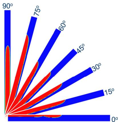
**Figure 6:** Taylor bubble shapes (red) for different inclinations. Red is gas and blue is liquid.
