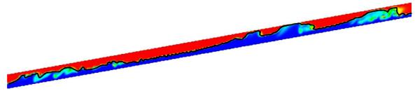
**Figure 11:** Excerpt of snap-shot from prediction of slug flow in an inclined pipe, 12 inches in diameter and 100 m long (the pipe diameter in the picture is magnified 5 times). The colours denote gas fraction, where red is 100% gas and deep blue is no gas (liquid). Flow is from left to right.
