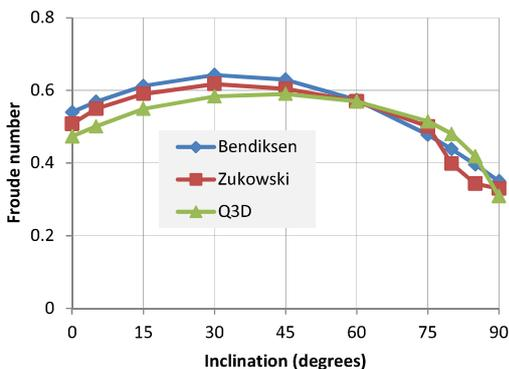
**Figure 7:** Comparison of Q3D results with experiments (Zukowski 1966) and correlation (Bendiksen 1984).
