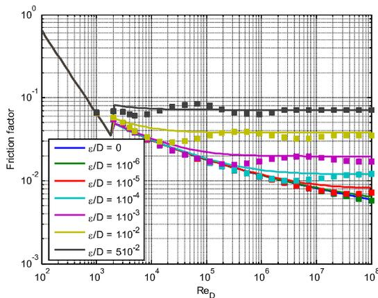
**Figure 2:** Moody diagram (Moody 1944) showing friction factor calculated using the Colebrook (1939) equation (lines) and Q3D (squares) for different relative wall roughnesses  $\epsilon/D$  versus pipe Reynolds number.
