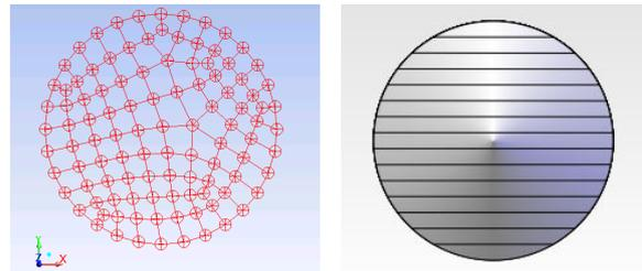
**Figure 3:** Mesh cross sections. Left: Fluent3D, Right: Q3D.
