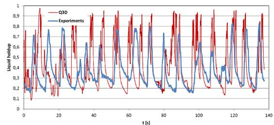
**Figure 12:** Liquid hold-up signal at a location 90 meters from the pipe inlet as compared to the experimental Gamma-ray signals.
