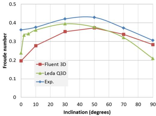
**Figure 5:** Comparison of experimental and CFD results for the Froude number, versus inclination angle. The pipe diameter is 76.2 mm.
