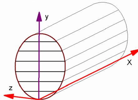
**Figure 1:** Quasi 3D grid cells, showing one axial (x-direction) and 7 vertical cells.
