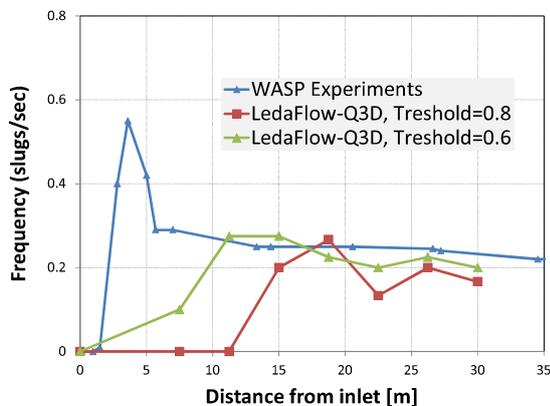
**Figure 10:** Slug frequency variation along the pipe.
