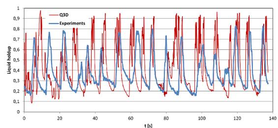
**Figure 12:** Liquid hold-up signal at a location 90 meters from the pipe inlet as compared to the experimental Gamma-ray signals.
