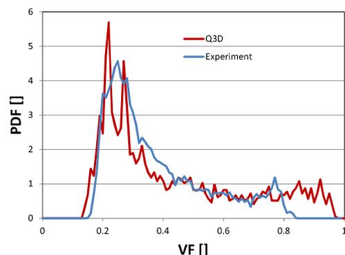
**Figure 13:** Probability density function (PDF) of the liquid volume fraction (VF) signal at 90 m from inlet compared with that of experimental data.
