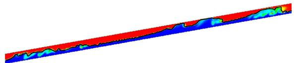
**Figure 11:** Excerpt of snap-shot from prediction of slug flow in an inclined pipe, 12 inches in diameter and 100 m long (the pipe diameter in the picture is magnified 5 times). The colours denote gas fraction, where red is 100% gas and deep blue is no gas (liquid). Flow is from left to right.
