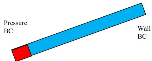
**Figure 4:** Initial state volume fraction with boundary conditions. Gas (red) is patched in at the bottom end of the liquid (blue) filled pipe. The pressure boundary is a pressure outlet with gas only backflow.
