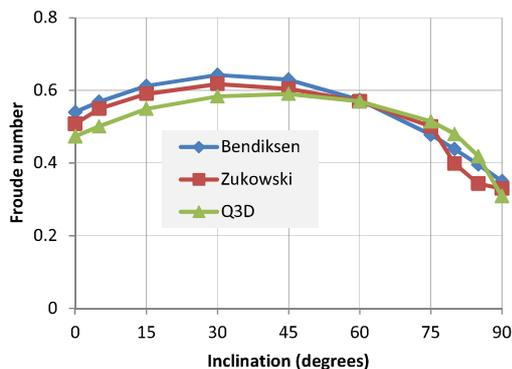
**Figure 7:** Comparison of Q3D results with experiments (Zukowski 1966) and correlation (Bendiksen 1984).
