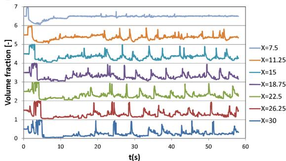
**Figure 9:** Liquid hold-up time-series for hydrodynamic slug flow at different locations ( $X$  [m]) along the horizontal pipe. Vertical axis is shifted by 1.0 for each series for readability.
