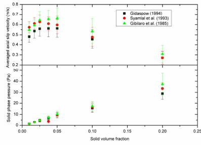
Figure 2. Comparison of averaged axial slip velocity and solid phase pressure obtained from different microscopic drag models.
