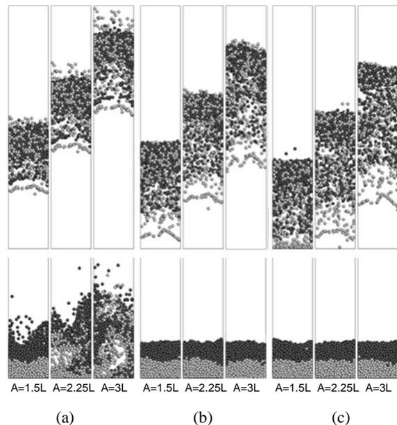
**Figure 4:** Solid flow patterns at maximum particle height in the first cycle for all variants of the trapezoidal profile (top) and snapshots at a rested state on completion of separation (bottom). Heavy and light particle are coloured grey and black respectively. (a)  $T=1$  s, (b)  $T=2$  s, (c)  $T=3$  s
