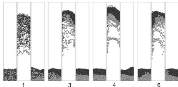
**Figure 2:** Solid flow patterns shown by particle position for variant  $T=2$  s,  $A=3$  L, at the: 1<sup>st</sup>, 3<sup>rd</sup>, 4<sup>th</sup>, and 6<sup>th</sup> cycle. Heavy and light particle are coloured grey and black respectively.
