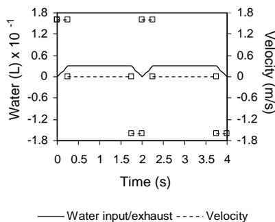
**Figure 1:** An example of the trapezoidal pulsation profile applied at inlet boundary condition.  $T=2$  s,  $A=3$  L
