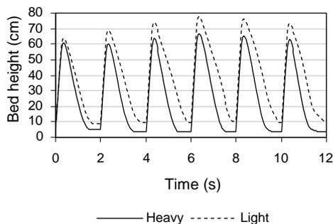
**Figure 3:** Mean particle position for variant  $T=2$  s,  $A=3$  L.
