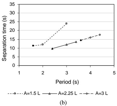
**Figure 6.** The effect of separation time against pulsation profile input parameters. (a) Volumetric input, (b) Cycle Period
