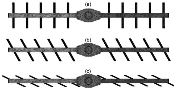
**Figure 3:** Example rake blade configurations, (a) 0°, (b) 30°, (c) 65°.
