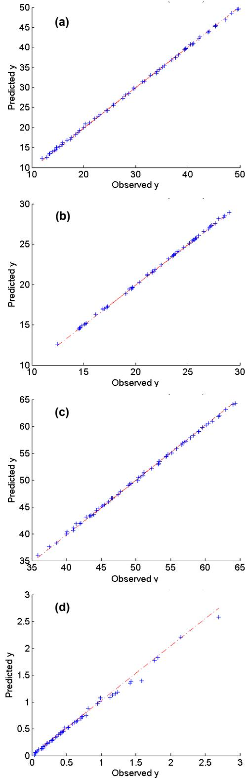
**Figure 7:** Cross-validated predictions versus actual values for (a) pressure component of torque, (b) viscous component of torque (c) total torque and (d) plug flow metric.
