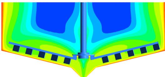
**Figure 5:** Residence time contours on a plane through the rake (rake speed 1.25 rpm, blade angle 30°). Ten linearly distributed colour bands of blue to red from 0 to 4000 s.
