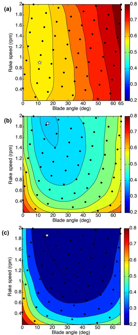
**Figure 8:** Contour plots showing the three different objective functions and the optimum value (white star) for (a) 80:20, (b) 50:50 and (c) 20:80 preference to torque and plug flow metric, respectively.
