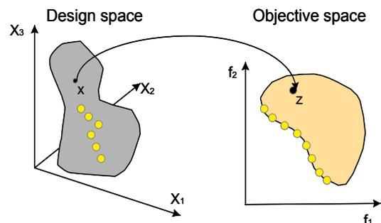
**Figure 9:** Representation of the design variable space and the corresponding objective space.
