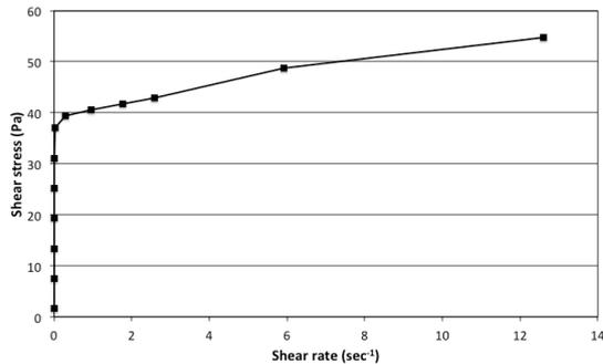
**Figure 4:** Rheogram of shear stress versus strain rate for the slurry used in the simulations.
