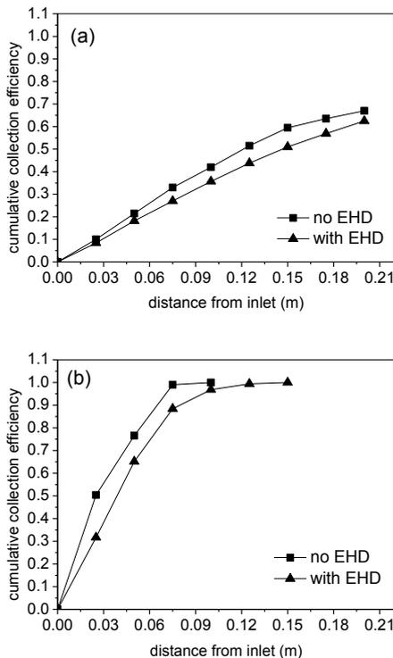
Figure 5: Cumulative collection efficiency for  $V=40$  kV and  $d_p=1.5$   $\mu$ m: (a)  $u_0=1.8$  m/s; (b)  $u_0=0.3$  m/s
