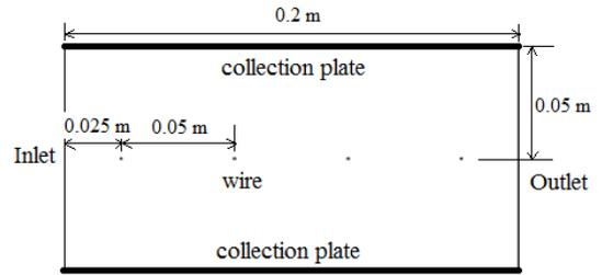
Figure 2: Simulation domain and its dimensions
