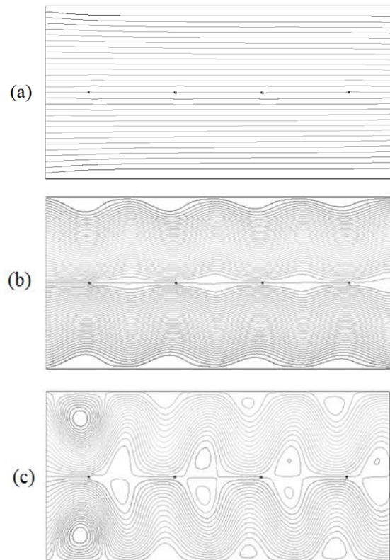
Figure 3: Flow streamlines for various  $N_{EHD}$ : (a) 0; (b) 10.3; (c) 15.6:
