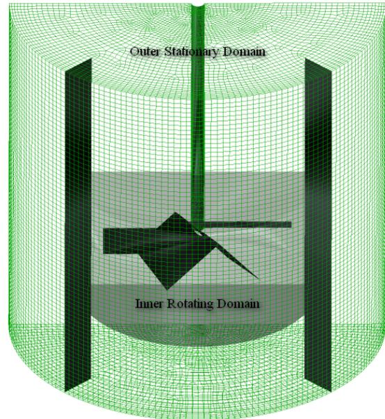
**Figure 1:** Computational domain and grid distribution in stirred tank
