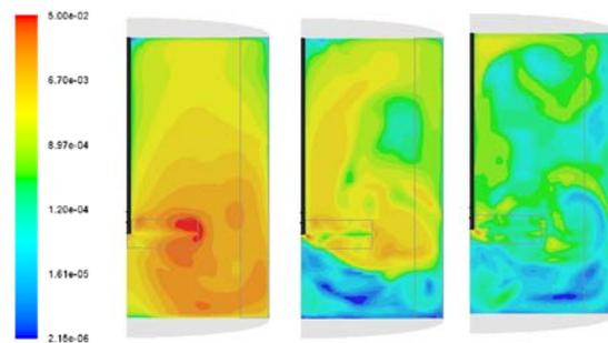
**Figure 6:** Normalised turbulent kinetic energy contours at mid-baffle plane for  $N = N_{js}$  of (a) single phase, (b) solid phase (20 wt%) and (c) solid phase (40 wt%).
