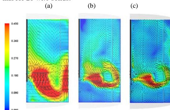
**Figure 4:** Normalised velocity maps and velocity vectors at mid-baffle plane for  $N = N_{js}$  of (a) single phase, (b) solid phase (20 wt%) and (c) solid phase (40 wt%).
