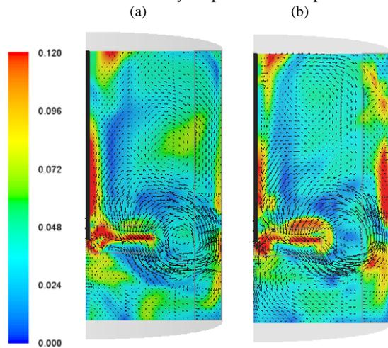
**Figure 5:** Normalised slip velocity maps and velocity vectors at mid-baffle plane for  $N = N_{js}$  of (a) 20 wt% solid and (b) 40 wt% solids.
