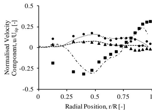
**Figure 2:** The three velocity components in a horizontal plane at  $z/H = 0.2$  for 20 wt% and  $N=N_{js}$ . ■ Experimental Axial Velocity — · — · Simulated Axial Velocity ▲ Experimental Radial Velocity — · — · Simulated Radial Velocity ● Experimental Tangential Velocity ······· Simulated Tangential Velocity
