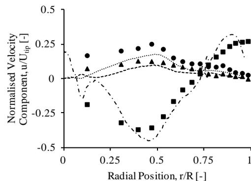
**Figure 3:** The three velocity components in a horizontal plane at  $z/H = 0.2$  for 40 wt% and  $N=N_{js}$ . ■ Experimental Axial Velocity — · — · Simulated Axial Velocity ▲ Experimental Radial Velocity — · — · Simulated Radial Velocity ● Experimental Tangential Velocity ······· Simulated Tangential Velocity
