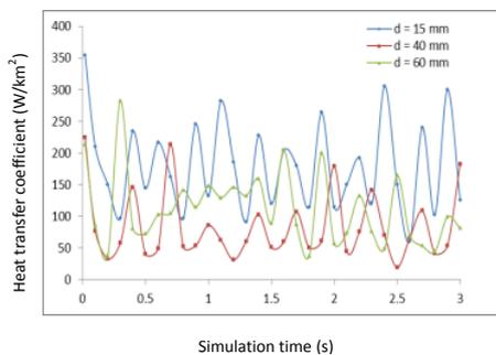
**Figure 8:** Evolution of heat transfer coefficients for different bed thicknesses
