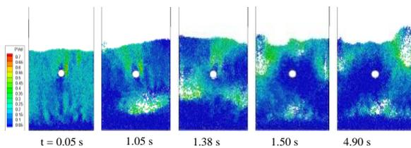
**Figure 3:** Solids flow patterns for pseudo-2D model
