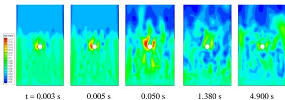
**Figure 5:** Wall shear stress for pseudo-2D model
