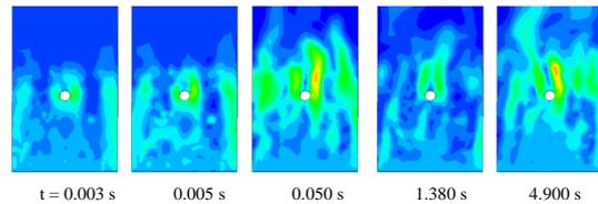
**Figure 6:** Wall shear stress for 3D model
