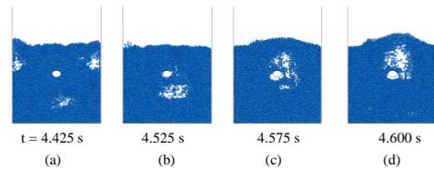
Figure 1: Snapshot of bubble transit past the cylinder
