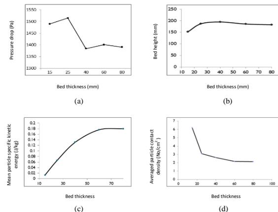
Figure 2: Sensitivity of (a) pressure drop, (b) bed height, (c) particle kinetic energy, and (d) particle-cylinder contact density on bed thickness
