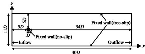
**Figure 2:** Flow around a square cylinder configuration.
