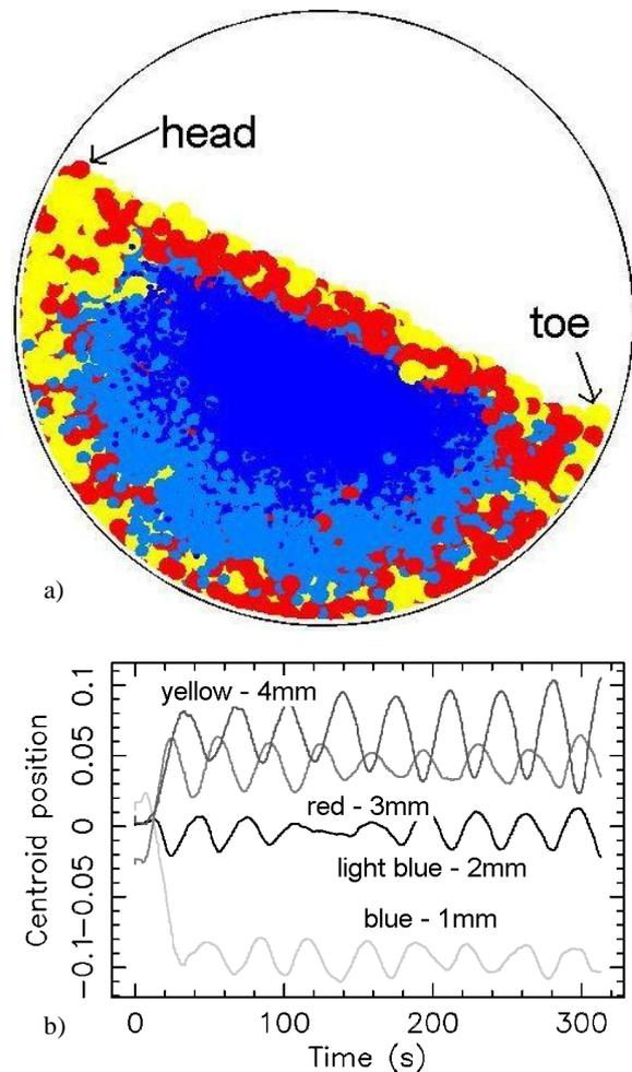
**Figure 5:** (a) Stable segregation pattern in a rotary classifier for a 4-component mixture with 4 mm (blue), 3 mm (blue), 2 mm (red) and 1 mm (yellow) particles. (b) Radial centroid variation for each size as a function of time. In (a) we also point out the head and toe of the bed, for later discussion.
