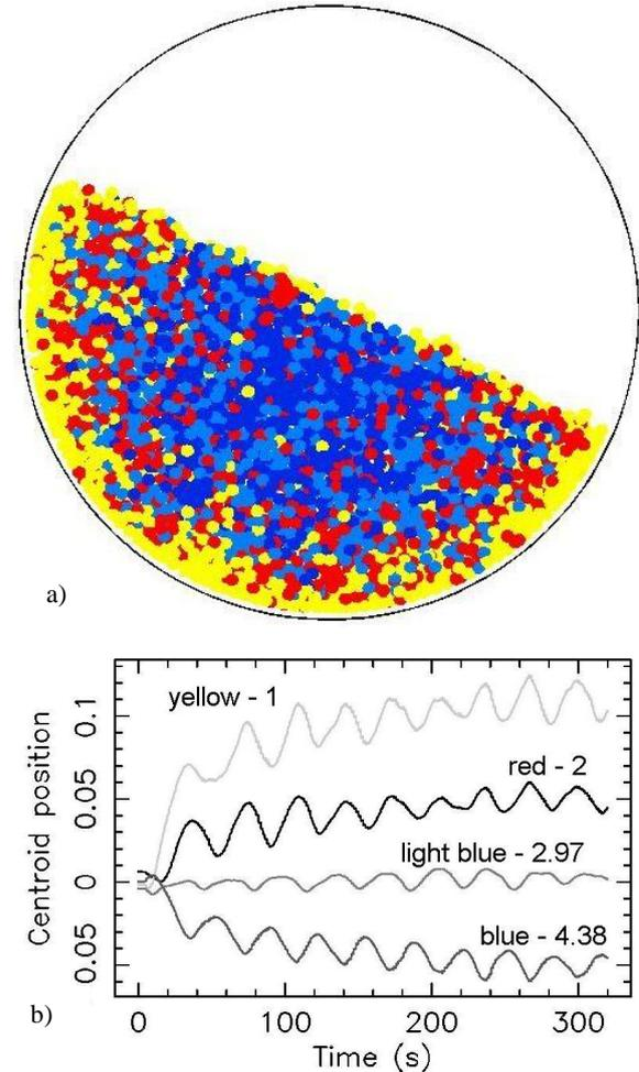
**Figure 2:** (a) Particle distribution at 305 secs and (b) radial centroid values, as a function of time for a 4 component density mixture. Densities are 1 (yellow particles), 2 (red) 2.97 (light blue) and 4.38 (blue).
