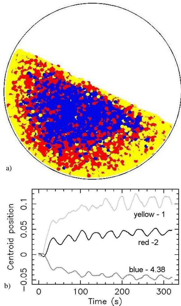
**Figure 1:** (a) Particle distribution at 305 secs and (b) radial centroid values, as a function of time for a 3 component density mixture. Density are 1.0 (yellow particles), 2.0 (red) and 4.38 (blue).
