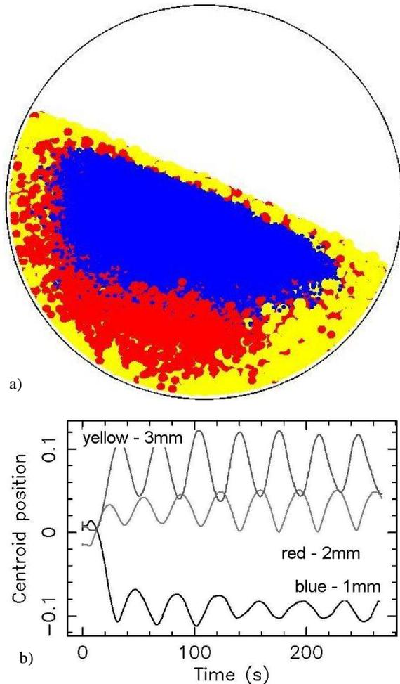
**Figure 4:** (a) Particle distribution at 300 secs and (b) radial centroid values, as a function of time for a 3-particle-sized mixture. Particles sizes are 1 mm (blue), 2 mm (red) and 3 mm (yellow) particles.
