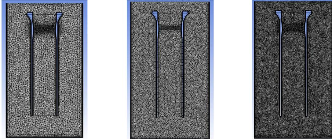
**Figure 2:** The computational mesh used (a) Coarse mesh (840 k elements), (b) Medium mesh (2 million elements), (c) Fine mesh (4.6 million elements)
