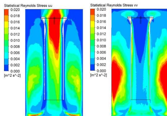
**Figure 6:** Normal stresses from fine mesh result with SST-SAS, highlighting anisotropic turbulence in annulus.
