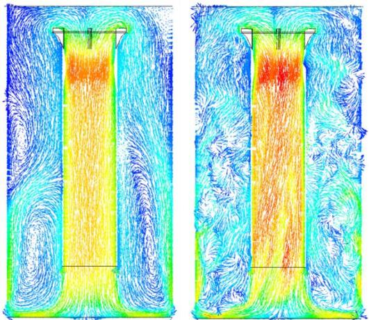
**Figure 8:** Instantaneous velocities (fine mesh) - SSG RSM (left) and SST-SAS (right) showing significant differences in dynamic flow behaviour.
