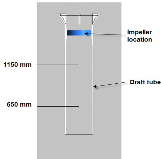
**Figure 1:** Laboratory-scale vessel geometry and LDV measurement positions.
