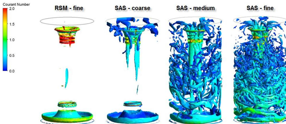
**Figure 5:** Iso-surface of Velocity Invariant  $Q$  at  $10^{-2} \text{ s}^{-2}$  showing the lack of turbulent structure resolved with RSM and the increasing structure resolved with SST-SAS as the mesh is refined.
