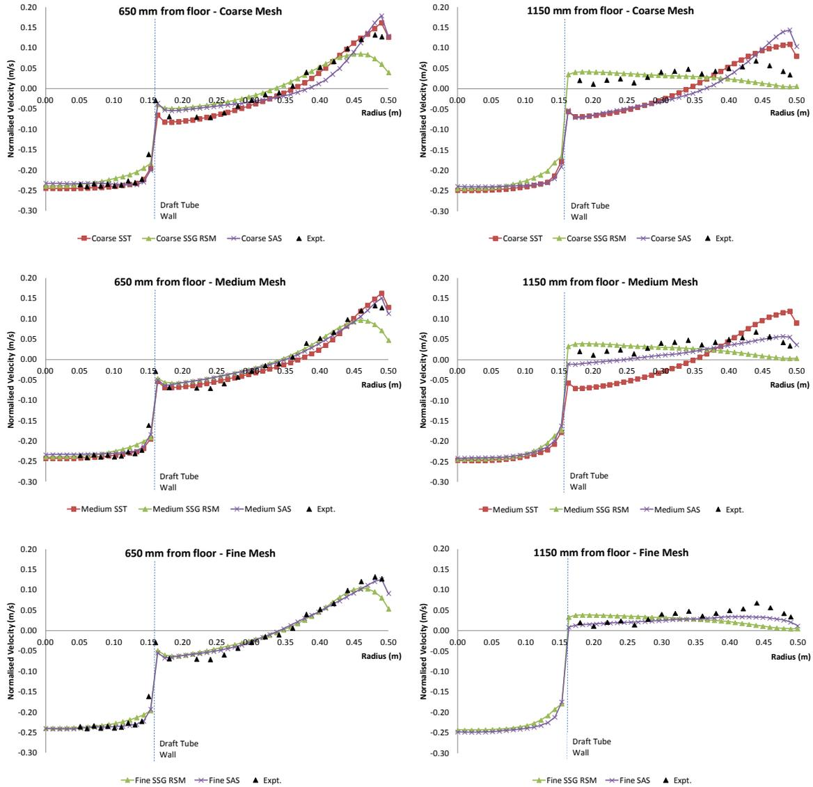
**Figure 3:** Velocity profiles on radial lines 650 mm and 1150 mm from floor of vessel with different mesh densities
