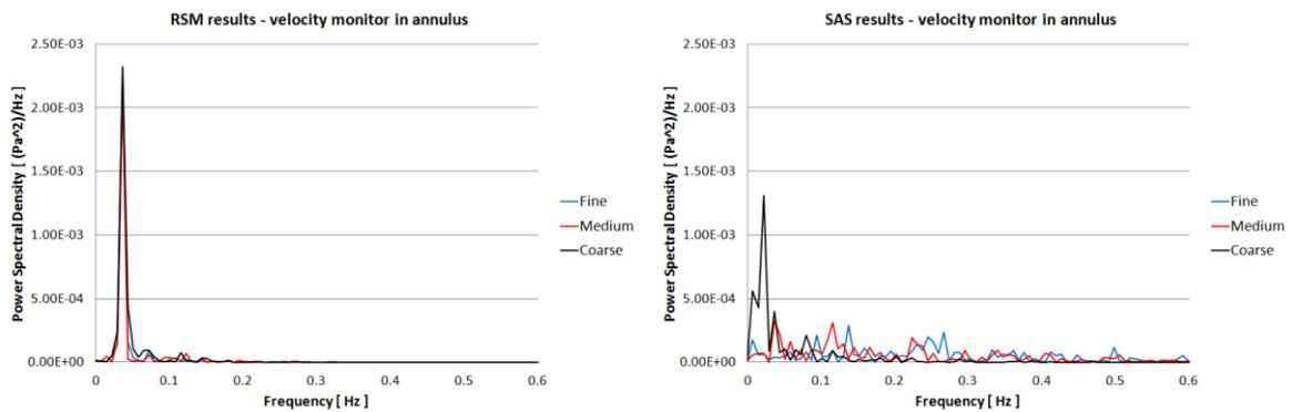
**Figure 4:** FFT analysis of fluctuating velocities at a point in the annulus; RSM runs (left) show a single dominant frequency on all meshes; SST-SAS runs (right) show increased spectral information as the mesh is refined.
