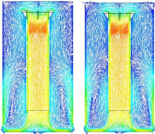
**Figure 7:** Transient average velocities (fine mesh) – SSG-RSM (left) and SST-SAS (right) showing very similar time-averaged behaviour.
