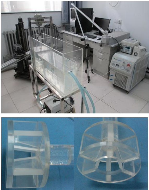
Figure 2: Experiment setup and impeller Furthermore, according to the results of stirred tank, the added baffles could increase the relative stirring velocity between the agitator and fluid and enhance the radial mixing, resulting in an improvement of mixing efficiency. In this paper, the effect of internal components on flow field in the mixer was analysed, such as four baffles and a plate covered on the top of mixer.
