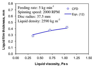
**Figure 9:** Influence of viscosity on film thickness.
