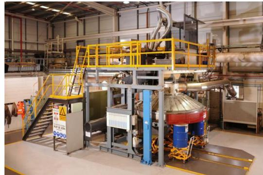
**Figure 1:** The semi-industrial scale (3 m in diameter) integrated dry granulation and heat recovery pilot plant at CSIRO.
