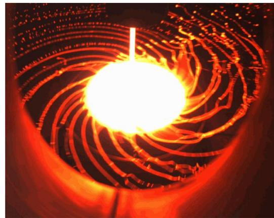
**Figure 2:** A typical still image from high speed video recording of the slag atomisation by a spinning disc in CSIRO's dry slag granulation process.
