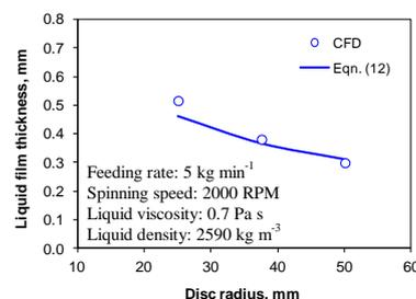
**Figure 8:** Influence of disc radius on film thickness.
