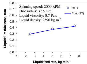
**Figure 6:** Influence of feeding rate on film thickness.
