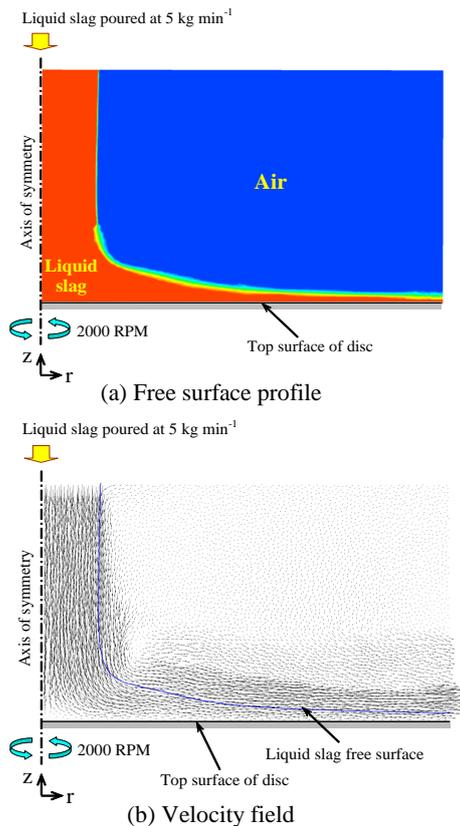
**Figure 5:** Predicted (a) liquid slag free surface profile and (b) velocity field for feeding rate:  $5 \text{ kg min}^{-1}$ , spinning speed: 2000 RPM, disc radius: 25 mm.
