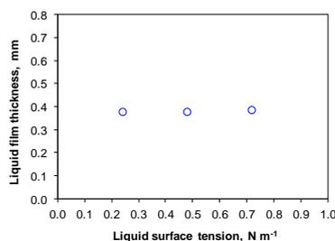
**Figure 11:** Influence of surface tension on film thickness. (Feeding rate:  $5 \text{ kg min}^{-1}$ , Spinning speed: 2000 RPM, Disc radius: 37.5 mm, Viscosity: 0.7 Pa s, Density:  $2590 \text{ kg m}^{-3}$ )
