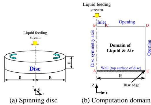
**Figure 3:** Schematic diagrams of three-dimensional disc geometry and two-dimensional computational domain.
