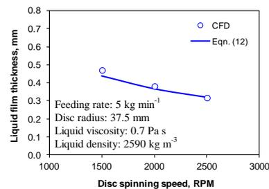
**Figure 7:** Influence of spinning speed on film thickness.
