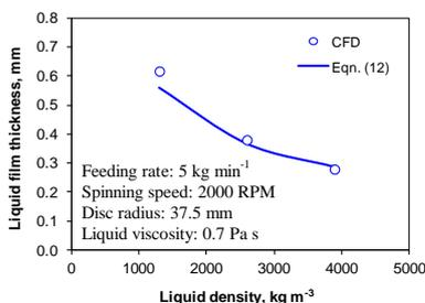
**Figure 10:** Influence of density on film thickness.
