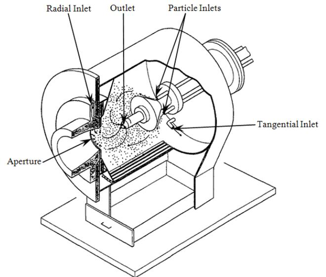
**Figure 2:** Schematic diagram of the reactor of Meier et al. (1996) chosen for model validation.
