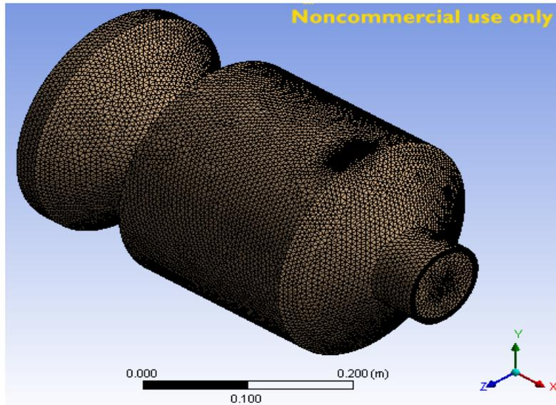
**Figure 4:** Mesh of the model of the Meier reactor.
