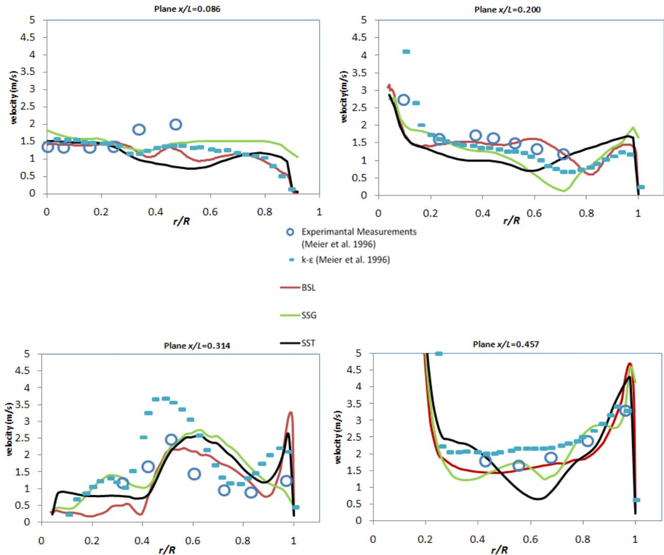
**Figure 7:** Comparison of CFD predictions with experimental data along four radial traverses, where  $r$  is the radial distance from initial point and  $R$  is the radius of the reactor, 125mm.
