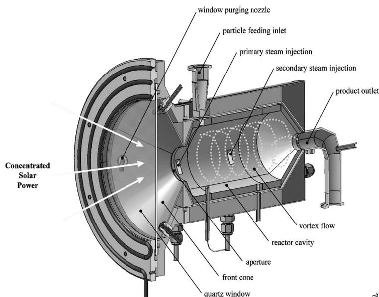
Figure 1: A scheme diagram of the solar vortex gasifier (Z'Graggen et al., 2006).
