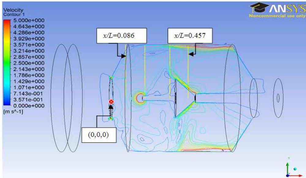
**Figure 6:** The locations of the four traverses and the predicted velocity contour in the reactor, where  $x$  defines as the distance from initial point to the traverses and  $L$  is 350 mm defined as the distance from initial point to the right end of the reactor.
