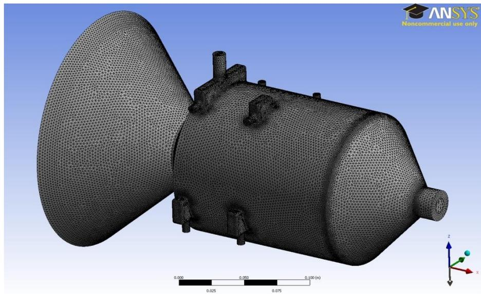
**Figure 5:** The unstructured mesh of Case 2.
