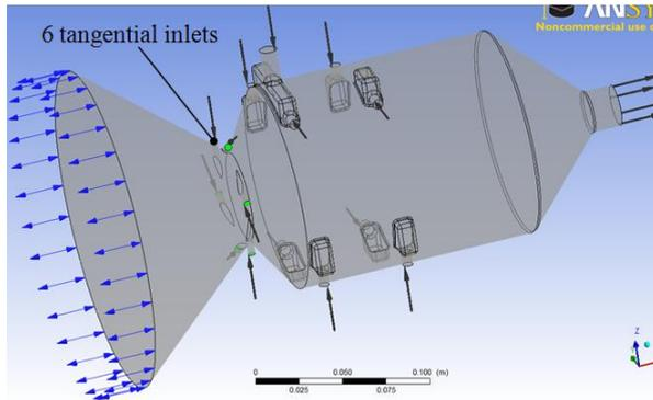
**Figure 4:** Six tangential inlets at the throat: Case 6.
