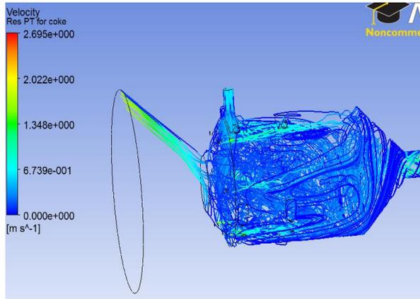
**Figure 9:** Trajectories of the injected particles in Case 4.
