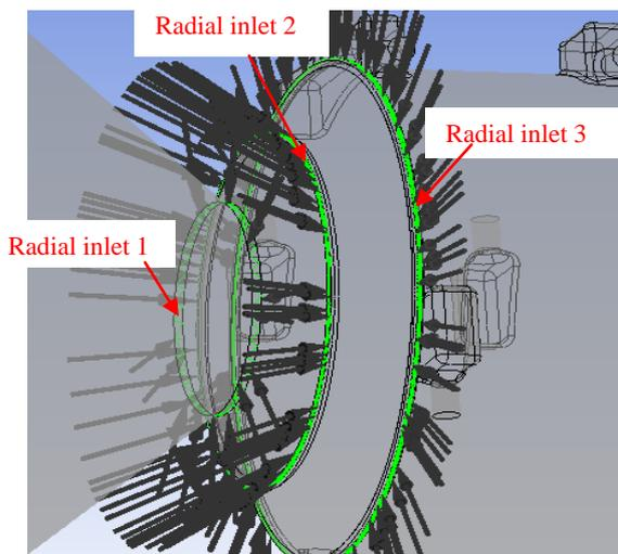
**Figure 2:** Radial gas inlets of Case 1 (Radial inlet 1), Case 2 (Radial inlet 2) and Case 3 (Radial inlet 3).
