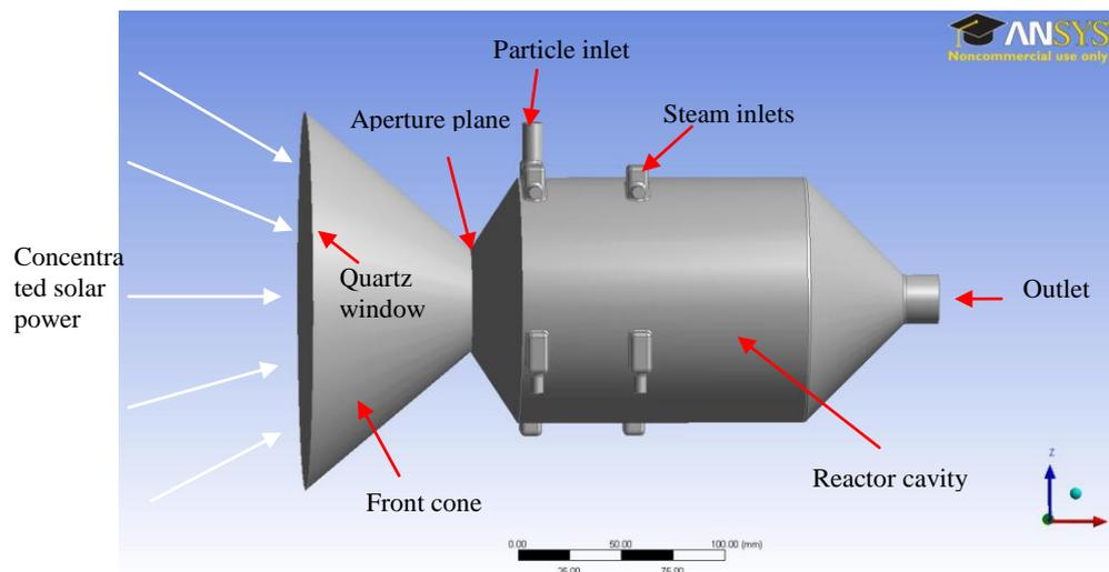
**Figure 1:** Geometric configuration of the Solar-enhanced Vortex Gasifier (SVG).
