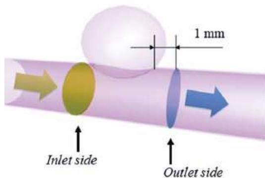
**Figure 2:** CFD Model of physical variable extraction site for defining energy loss
