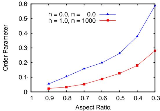
**Figure 4:** Orientational order parameter  $\chi_\theta$  for mono-disperse packings of oblate ellipsoids. Data is shown for the two extreme cases of zero inter-grain friction without a background fluid (blue triangles) and high inter-grain friction and high viscosity (red squares).
