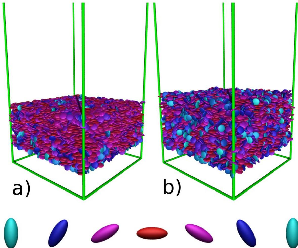
**Figure 3:** Images of packings of monodisperse oblate ellipsoids with an aspect ratio of 0.3 at the a) dense, and b) loose limits. Particles are coloured by the alignment of the grain with the horizontal axis as shown in the key.
