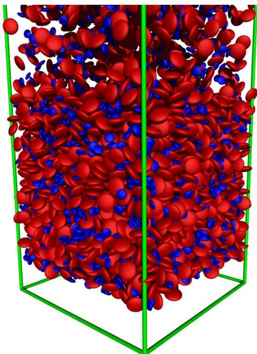
**Figure 8:** Image of the formation of a bi-disperse packing of oblate ellipsoids with aspect ratio of 0.4 and a volume ratio of 6:1.
