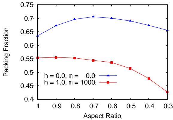
**Figure 2:** Packing fraction variation with aspect ratio for mono-disperse packings of oblate ellipsoids. Data is shown for the two extreme cases of zero inter-grain friction without a background fluid (blue triangles) and high inter-grain friction and high viscosity (red squares).
