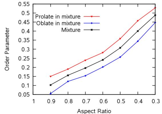
**Figure 6:** Variation in the orientational order parameter with aspect ratio for 50:50 mixture of oblate and prolate ellipsoids with the same aspect ratio. Packings were prepared with zero inter-grain friction without a background fluid.
