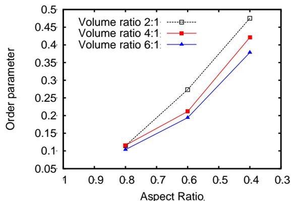
**Figure 10:** Variation in the orientational order parameter with aspect ratio for bi-disperse packings of ellipsoids.
