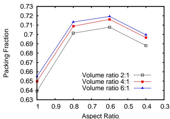
**Figure 9:** Packing fraction variation with aspect ratio for dense bi-disperse packings of oblate ellipsoids. Three particle volume ratios are shown. Packings were created with zero inter-grain friction and without a background fluid.
