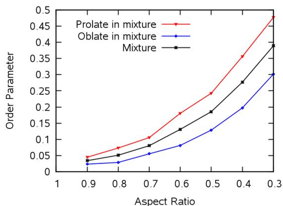
**Figure 7:** Variation in the orientational order parameter with aspect ratio for 50:50 mixture of oblate and prolate ellipsoids with the same aspect ratio. Packings were prepared with high inter-particle friction ( $\mu = 1000$ ) in a high viscosity fluid ( $\eta = 1.0$  Pa s).
