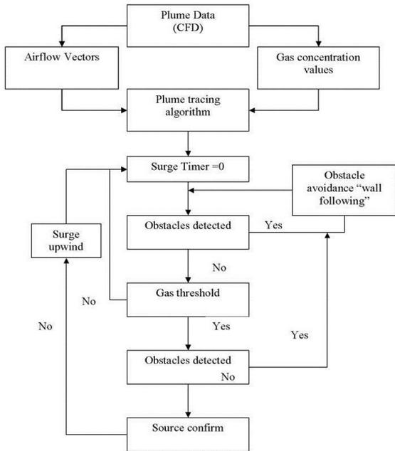
Figure 3: Plume tracing and source localization flow chart.
