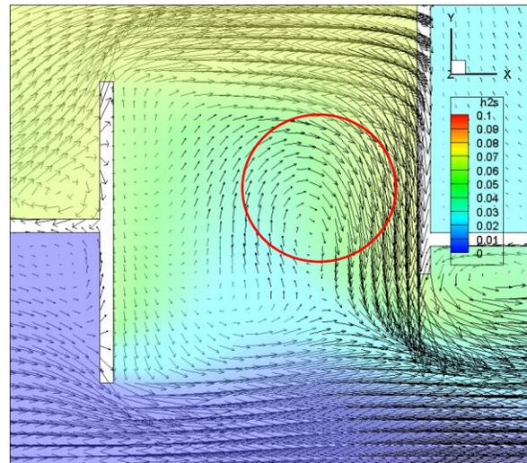
**Figure 8:** Effects of airflow vectors on robots heading when concentration drops below set threshold at height 1 m.
