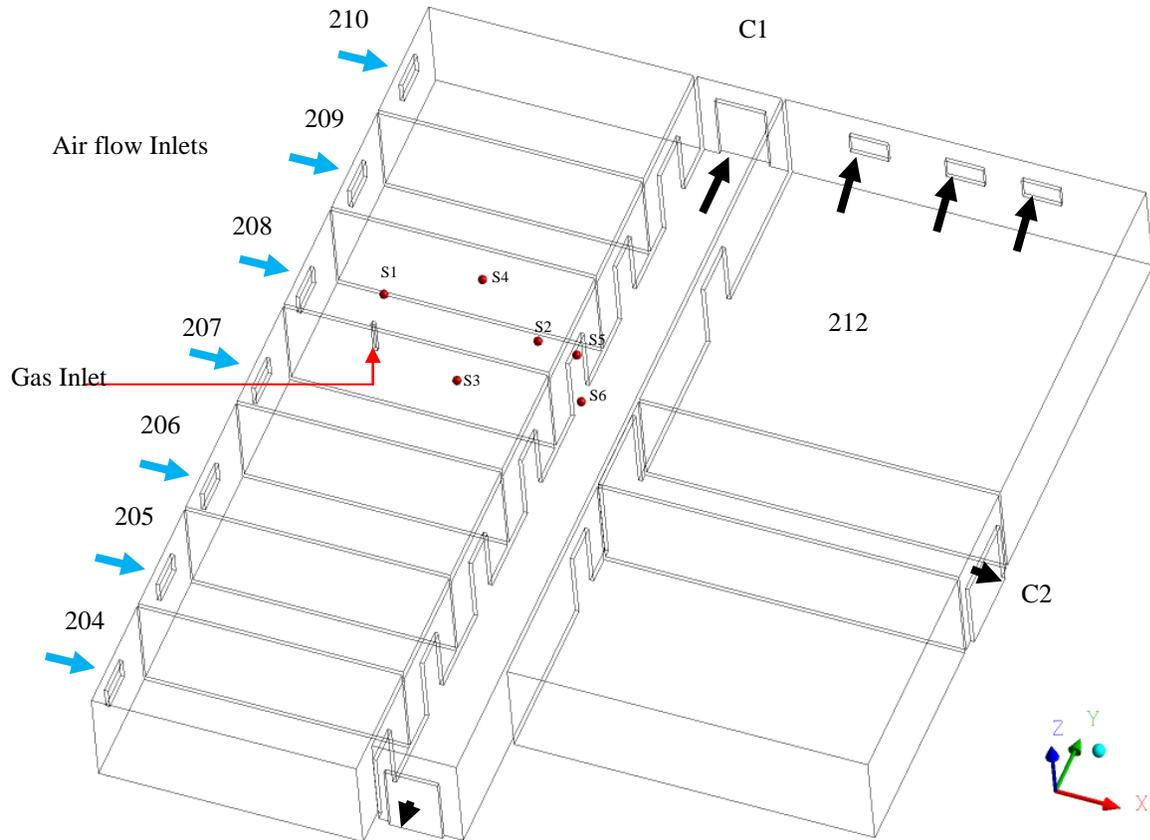
**Figure 1:** Simulation environment with arrows pointing towards the inlets of airflow, outlet mixture and location of the gas leak.
