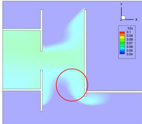
**Figure 7:** Concentration of H<sub>2</sub>S (% mass fraction) at the entrance of the suspected room at height 1 m.
