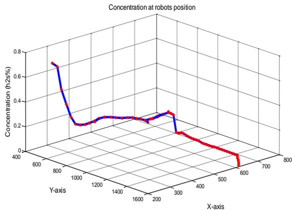
**Figure 10:** MATLAB simulation showing the concentration gradient trajectory set by the robot from the initial search till the highest point at the source.
