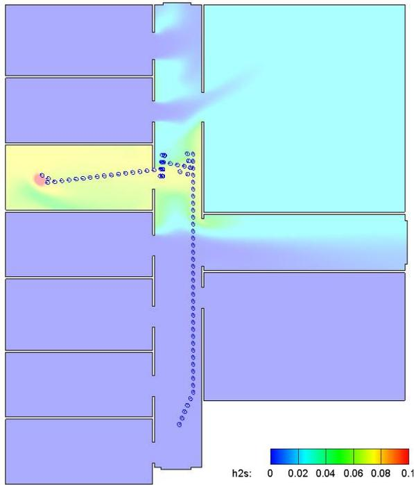
**Figure 9:** Top view of robots trajectory superimposed in a 3D search. The concentration contour is at the horizontal plane at height 1 m.
