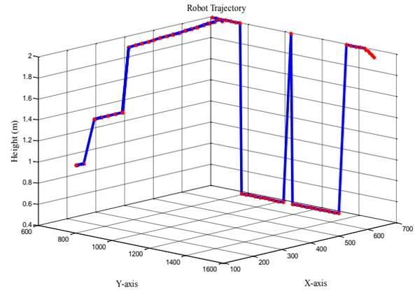
**Figure 11:** MATLAB simulation of the 3D plume search trajectory.
