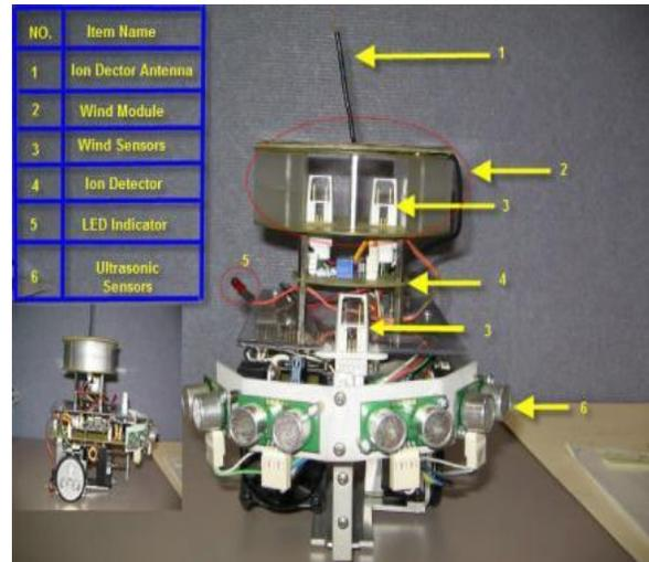
**Figure 2:** The physical robot used as a base for this study (Harvey et al., 2003)
