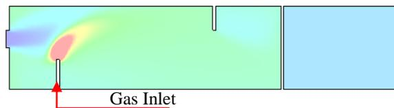
Figure 4: Side view (XZ) at  $Y=14.57$  m in room 208 showing the plume distribution.
