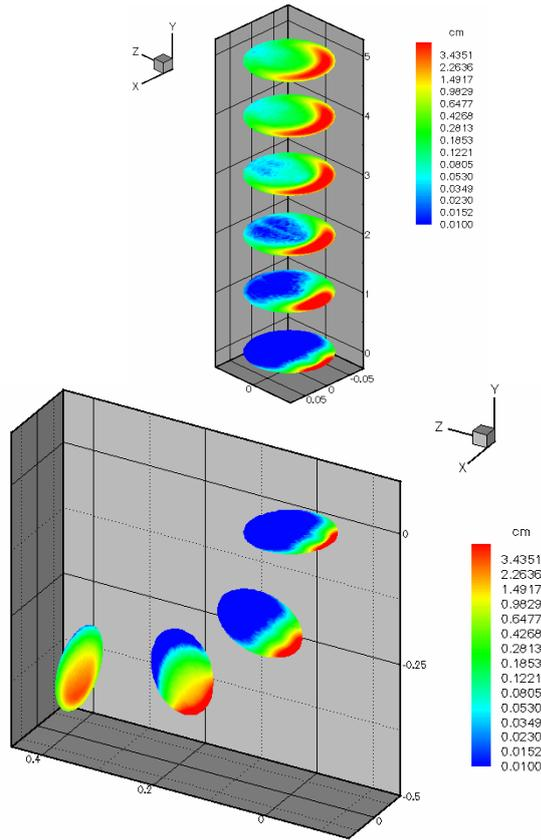
**Figure 11:** Cross-sectional distribution of particle concentration in  $\text{kg/m}^3$  along bend and vertical pipe ( $D = 150$  mm,  $U_0 = 27$  m/s,  $\eta = 1.0$ ,  $\Delta\gamma = 10^\circ$ , particle size distribution  $15 - 85$   $\mu\text{m}$ , four-way coupling).
