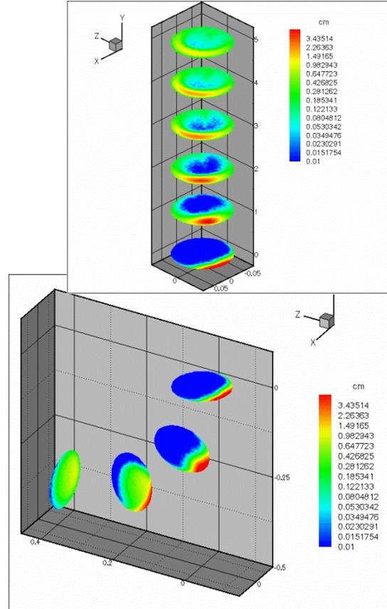
**Figure 12:** Cross-sectional distribution of particle concentration in  $\text{kg/m}^3$  along bend and horizontal pipe ( $D = 150$  mm,  $U_0 = 27$  m/s,  $\eta = 0.3$ ,  $\Delta\gamma = 10^\circ$ , particle size distribution  $15 - 85$   $\mu\text{m}$ , four-way coupling).
