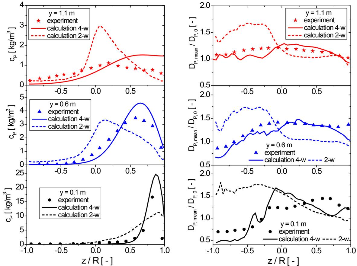
**Figure 2:** Profiles of particle concentration (left) and particle mean number diameter (right) downstream of the bend exit, comparison of calculations with experiments ( $D = 80$  mm,  $R_{\text{bend}} = 0.203$  m,  $U_0 = 14$  m/s,  $\eta = 0.5$ ,  $\Delta\gamma = 10^\circ$ , four-way coupling, particle size distribution  $15 - 85$   $\mu\text{m}$ ,  $St_{\text{bend}} = 0.076 - 2.445$ ).
