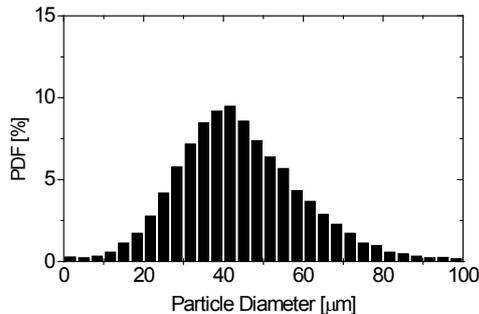
**Figure 1:** Size distribution of spherical glass beads (relative number frequency) used in the experiments of Huber and Sommerfeld (1998).
