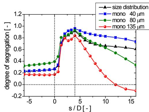
**Figure 9:** Non-dimensional segregation parameter along the pipe system for the cases 1 to 4 in Table 2 (size distribution Fig. 4 right, mono-sized  $40 \mu\text{m}$  Fig. 5, mono-sized  $80 \mu\text{m}$  Fig. 6, mono-sized  $135 \mu\text{m}$  Fig. 7 ( $D = 150 \text{ mm}$ ,  $U_0 = 27 \text{ m/s}$ ,  $\eta = 0.3$ ,  $\Delta\gamma = 10^\circ$ , bend radius 2.54 pipe diameters, four-way coupling).
