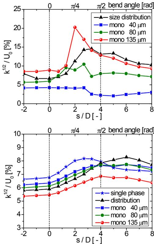
**Figure 10:** Fluctuating energy along the extended pipe bend; top) particle-phase, bottom) gas-phase ( $D = 150$  mm,  $U_0 = 27$  m/s,  $\eta = 0.3$ ,  $\Delta\gamma = 10^\circ$ , bend radius 2.54 pipe diameters, four-way coupling, different particle sizes).
