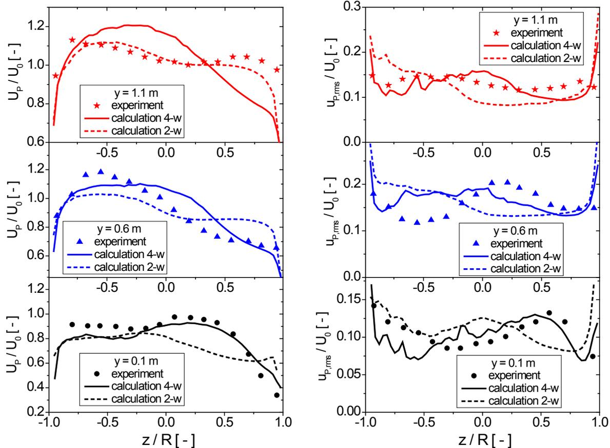
**Figure 3:** Profiles of vertical particle velocity (left) associated rms-value (right) downstream of the bend exit, comparison of calculations with experiments ( $D = 80$  mm,  $R_{\text{bend}} = 0.203$  m,  $U_0 = 14$  m/s,  $\eta = 0.5$ ,  $\Delta\gamma = 10^\circ$ , four-way coupling, particle size distribution  $15 - 85$   $\mu\text{m}$ ,  $St_{\text{bend}} = 0.076 - 2.445$ ).
