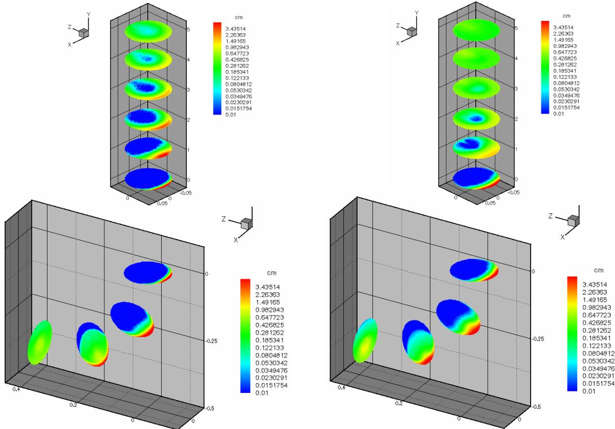
**Figure 6:** Cross-sectional distribution of particle concentration in  $\text{kg}/\text{m}^3$  along bend and vertical pipe ( $D = 150$  mm,  $U_0 = 27$  m/s,  $\eta = 0.3$ ,  $\Delta\gamma = 10^\circ$ , four-way coupling, mono-sized 40  $\mu\text{m}$ )
