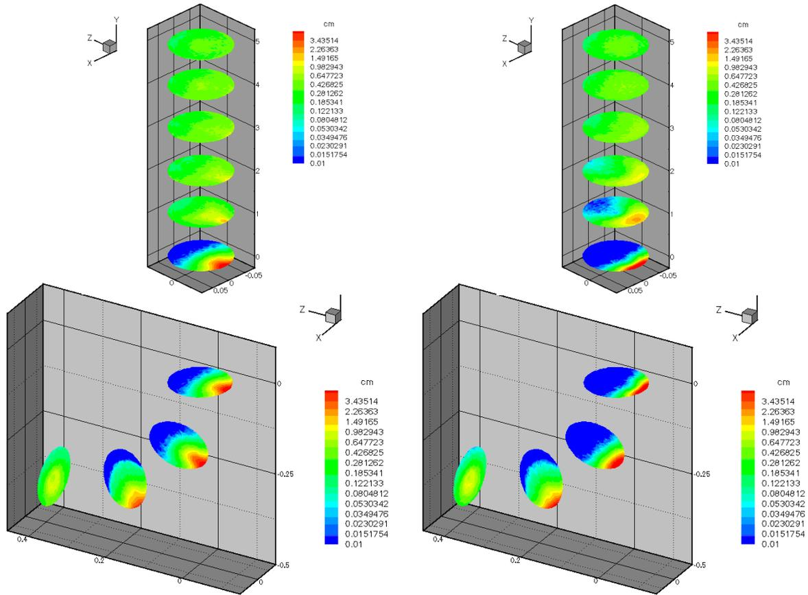
**Figure 5:** Cross-sectional distribution of particle concentration in  $\text{kg/m}^3$  along bend and connecting vertical pipe: left) two-way coupling, right) four-way coupling ( $D = 150$  mm, bend radius 2.54 pipe diameters,  $U_{av} = 27$  m/s,  $\eta = 0.3$ ,  $\Delta\gamma = 10^\circ$ , particle size distribution 15 – 85  $\mu\text{m}$ ).
