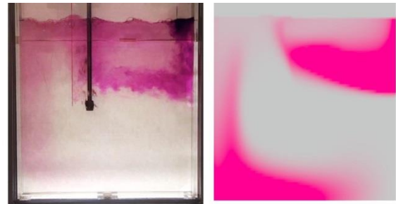
Figure 8: Evolution of tracer concentration in Case 2 for experiment (left) and simulation (right) 11 seconds after tracer injection
