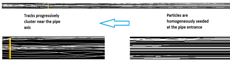
Figure 8: Low-Stokes (4.24) particle tracks clustering in the neighbourhood of the pipe axis. Particle/carrier density ratio = 13.3.
