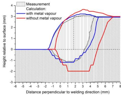
**Figure 4:** Comparison of measured weld cross-sections with those predicted by the computational model. Predictions of the model including and excluding the influence of metal vapour are shown. The original metal profile is shown by the broken line. The parameters are as given in Table 1, except for arc current 104 A, welding speed 10 mm s<sup>-1</sup> and wire feed rate 78 mm s<sup>-1</sup>.
