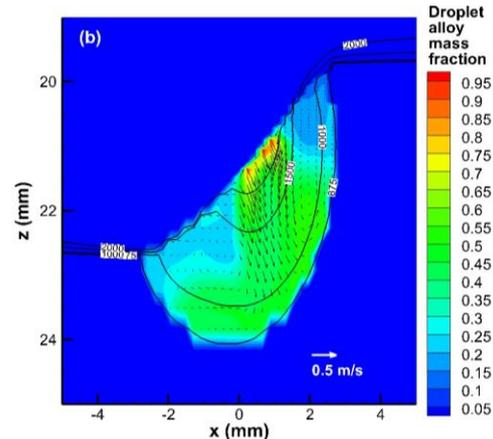
**Figure 3:** Fraction of the droplet alloy in a cross-section of the weld pool, for the  $y = 0.2$  mm plane. Velocity vectors, and temperature contours for 875, 1000, 1500 and 2000 K are also shown.
