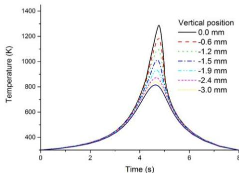
**Figure 7:** Thermal history at different vertical ( $z$ ) positions at  $x = 0$ . The  $x$  and  $z$  coordinates correspond to those used in Figure 4.
