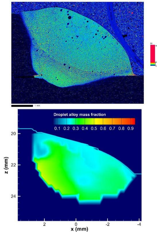
**Figure 5:** Measured silicon mass fraction in a cross-section of the weld (top) and calculated mass fraction of the droplet alloy (bottom). The scale in the top image runs from 0% Si (black) to 6.6% Si (red).
