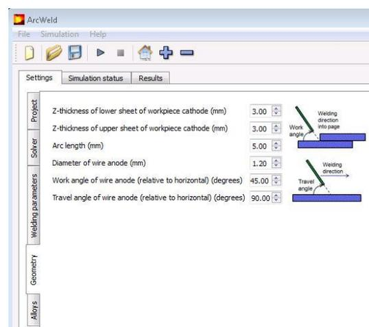
**Figure 6:** View of the graphical user interface, showing the geometry input window.
