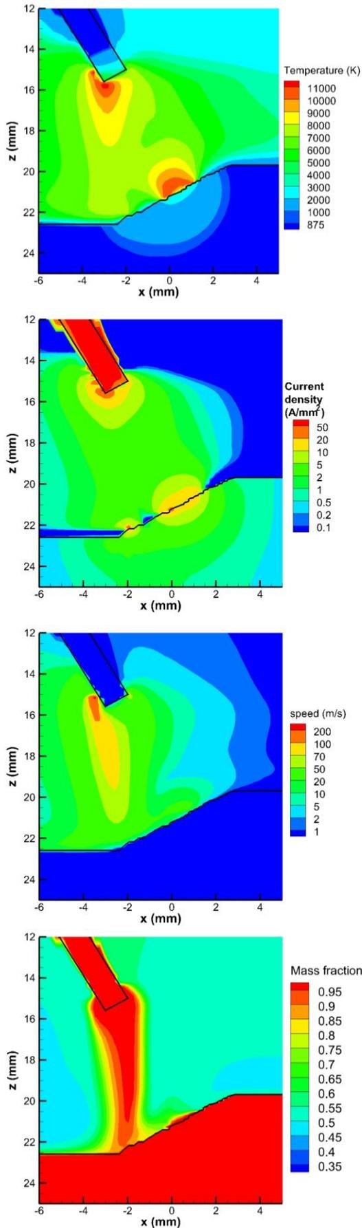
**Figure 2:** Distributions of temperature, current density, flow speed and aluminium vapour mass fraction in the vertical plane through the wire electrode.
