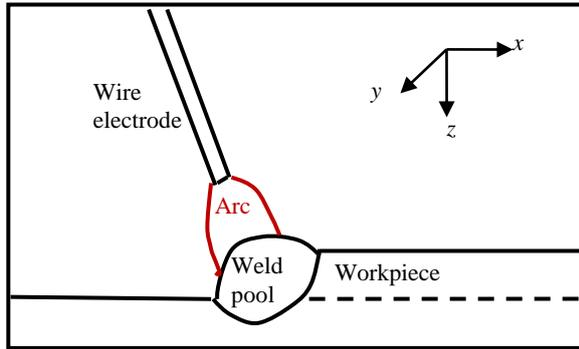
**Figure 1:** Schematic showing a cross section of the computational domain.
