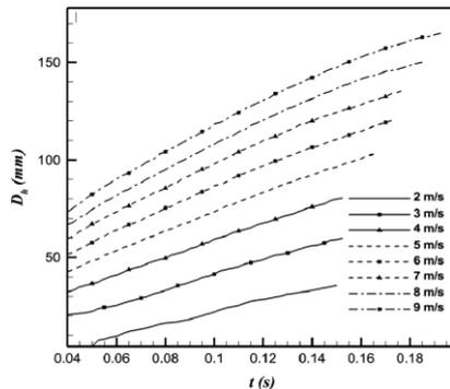
**Figure 6:** CFD prediction of bubble growth with gas injection rate for central injection (Kumar et al., 2013)
