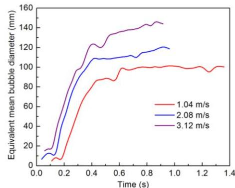
**Figure 7:** Variation of bubble size with gas injection rate for asymmetric injection
