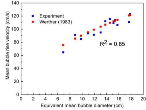
**Figure 4:** Experimental validation of the bubble characteristics with Werther's correlation
