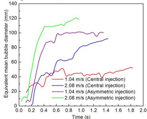
**Figure 8:** Effect of jet position on the bubble size variation with gas injection rate
