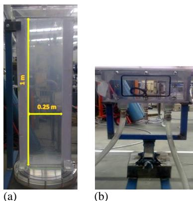
**Figure 1:** 2D Fluidized bed (a) column, (b) wind box
