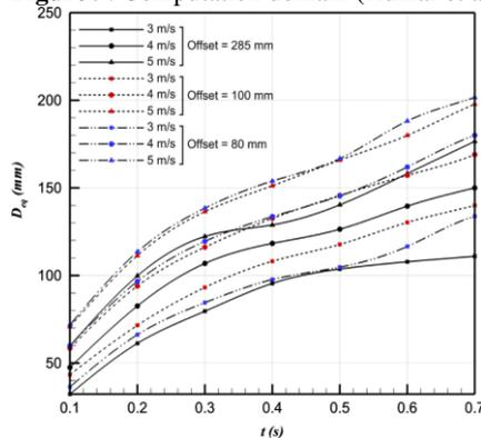
**Figure 10:** Variation of equivalent bubble diameter with gas injection rate for three different wall offsets (Kumar et al., 2013)
