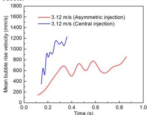
**Figure 14:** Effect of jet position on the variation of bubble rise velocity with gas injection rate
