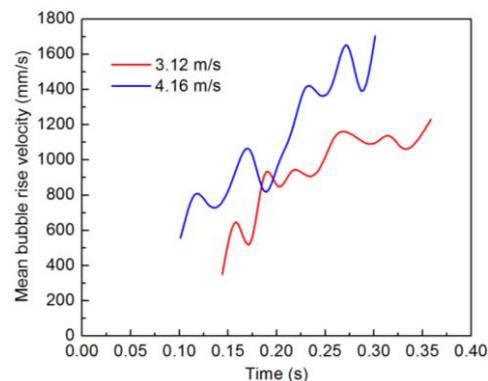
**Figure 13:** Effect of gas injection rate on bubble rise velocity for central injection
