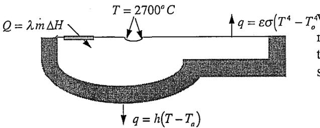
Figure 3: Temperature Field Boundary Conditions
