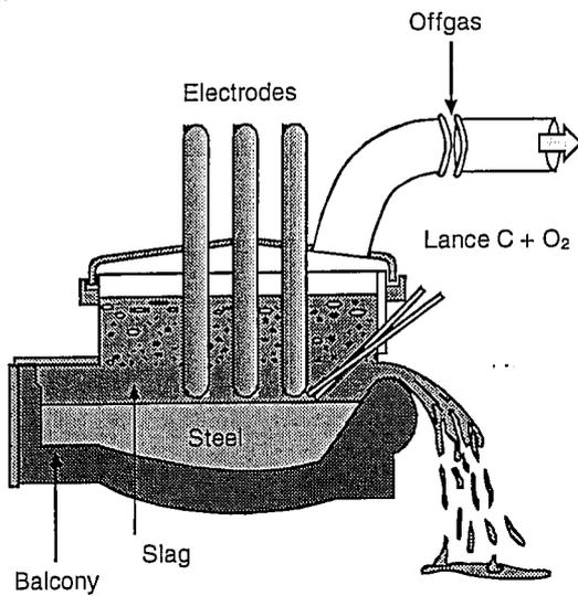
Figure 1: Diagram of an EAF
