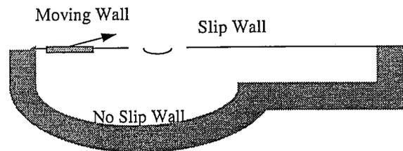
Figure 2: Flow Field Boundary Conditions
