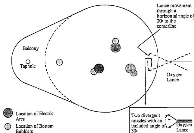
Figure 4: Layout of Oxygen Lance, Electric Arcs and Bottom Bubblers
