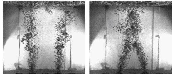
**Figure 3** : 2 plumes configuration at different instants – flow-rate : 5l/min
