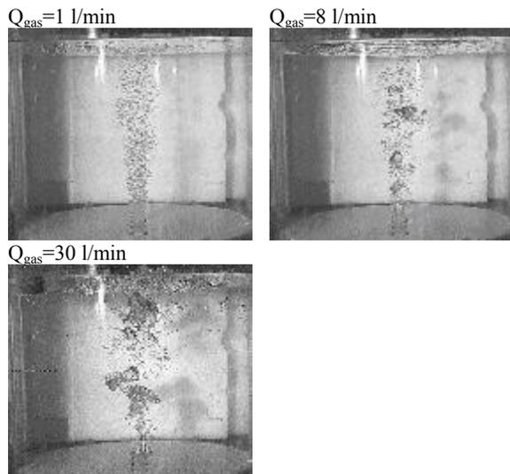
**Figure 1** : Plume behaviour for different air flow-rates.
