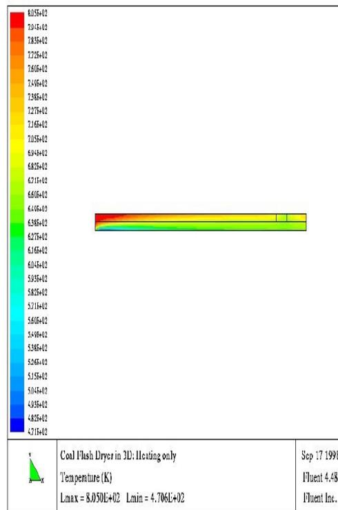
Figure 10: Temperature Distribution of Coal Particles
