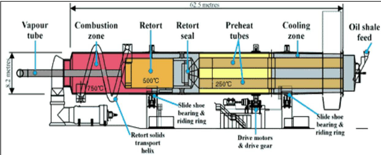
Figure 1: Cross Section of ATP
