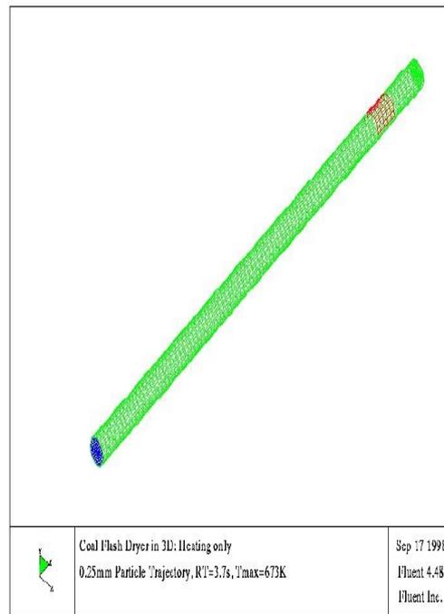
Figure 8: The Grid for Coal Drying Modelling
