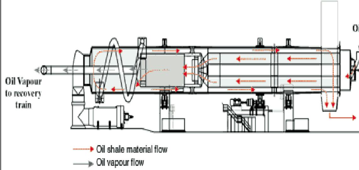
Figure 2: Material Flow through the ATP
