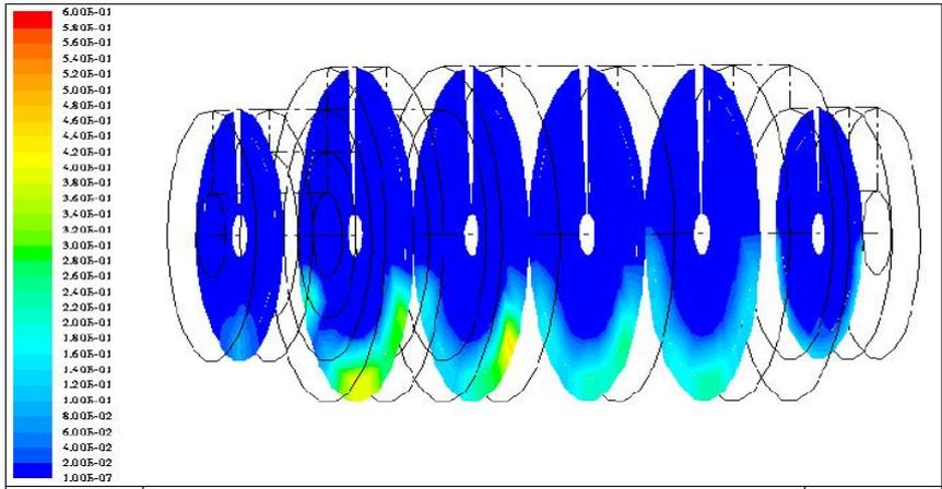
Figure 3: Oil Shale Volume Fraction
