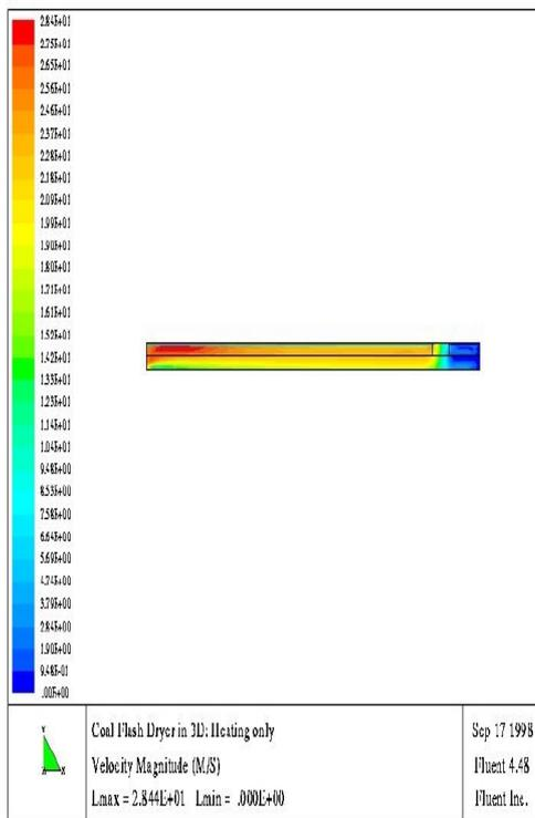
Figure 9: Velocity Contours of Coal Particles
