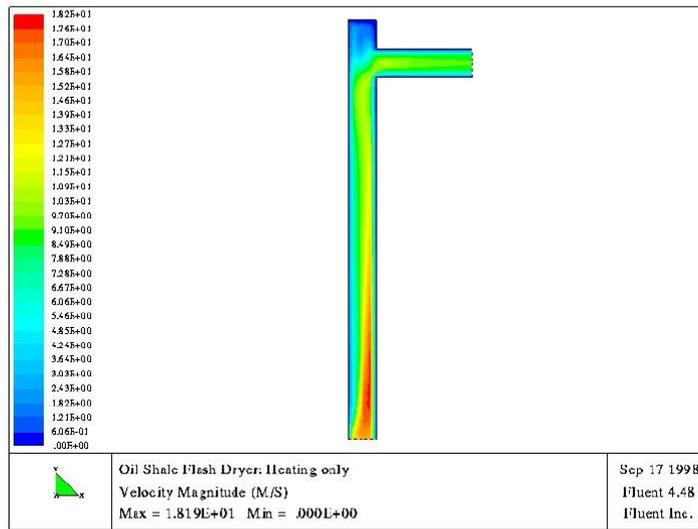
Figure 5: Velocity Contours
