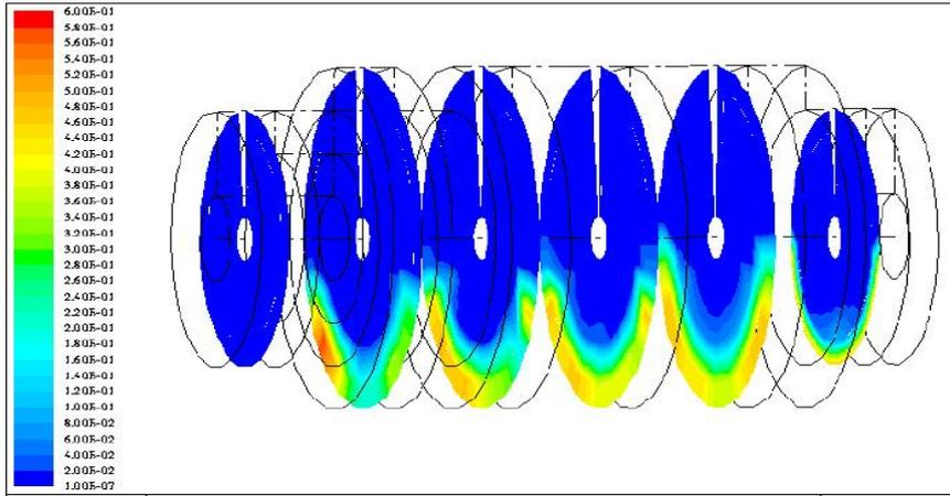
Figure 4: Retort Shale Volume Fraction
