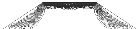
Figure 1: Contour diagram of mass fraction of oxygen in gas phase. Contour interval is 5% of total range (0 to 0.22).
