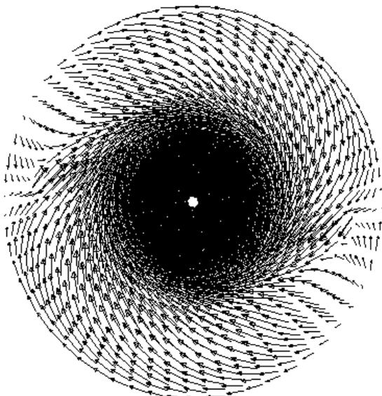
**Figure 9:** Velocity profile on bath surface (Baffles included).
