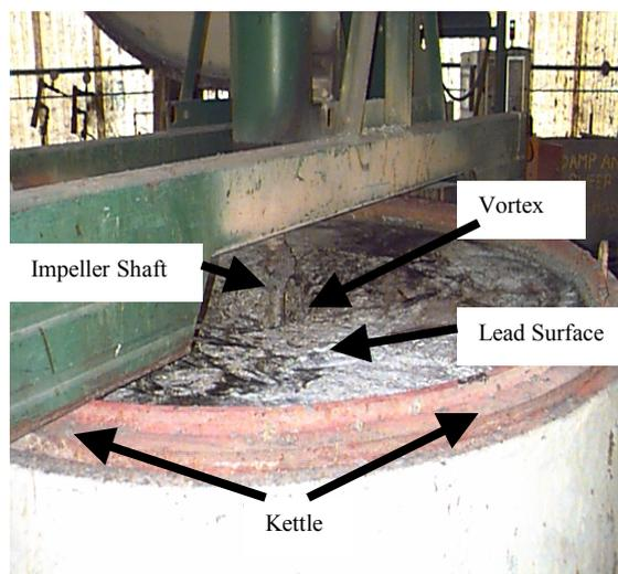
Figure 1: Lead refining operation using a kettle
