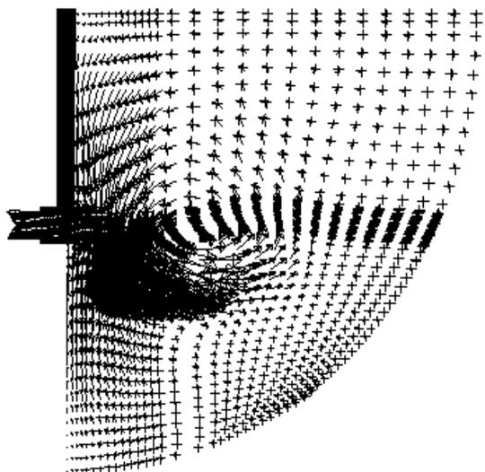
**Figure 8:** Flow profile in kettle (No Baffles).
