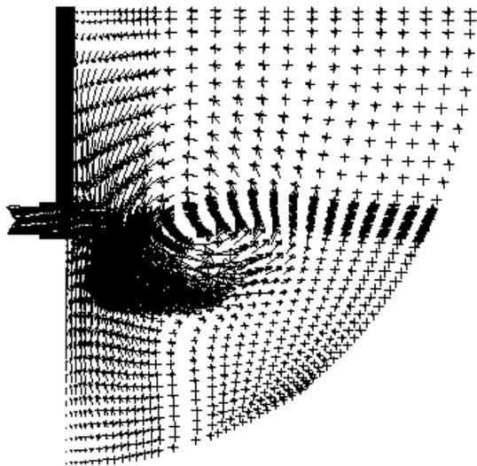
**Figure 8:** Flow profile in kettle (No Baffles).
