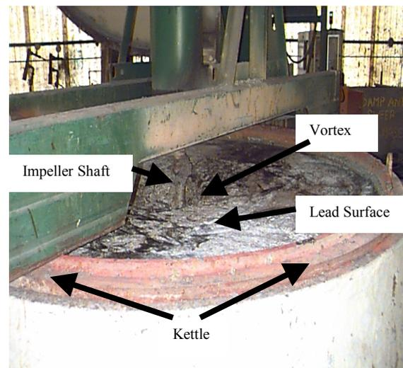
Figure 1: Lead refining operation using a kettle
