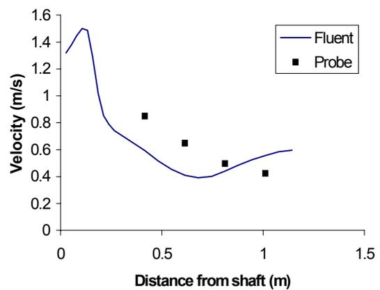
**Figure 14:** Velocity comparisons for sampling points on line (1) - (no baffles).
