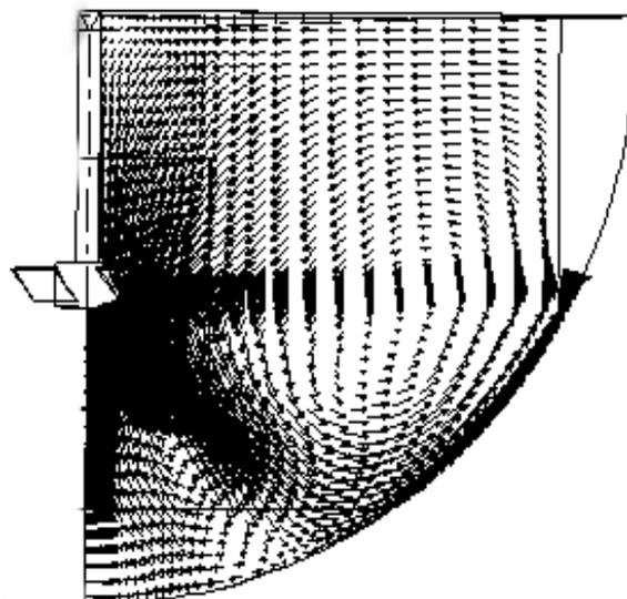
**Figure 10:** Flow profile in kettle (Baffles included).
