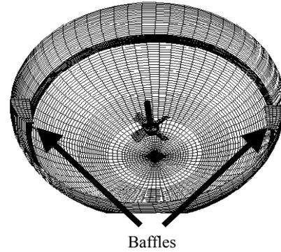
Figure 3: Kettle model with baffles.
