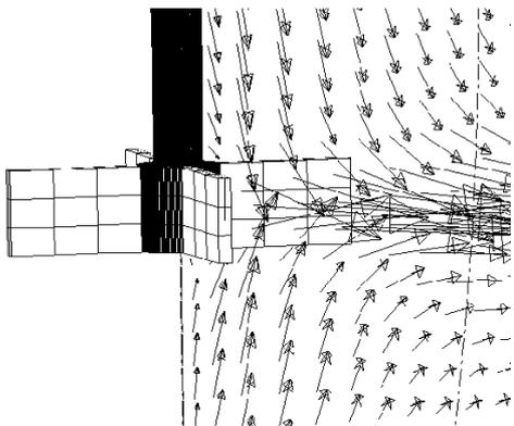
Figure 17: Velocity profile around impeller blades.
