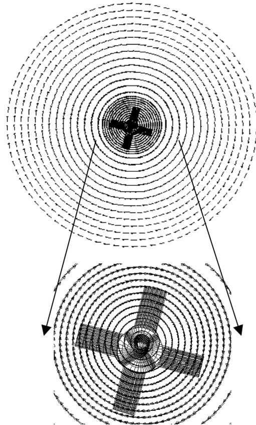
**Figure 7:** Flow profiles at top of kettle (No Baffles).
