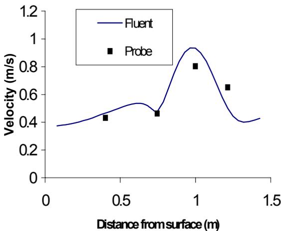
**Figure 13:** Velocity comparisons for sampling points on line (2) - (baffles included).
