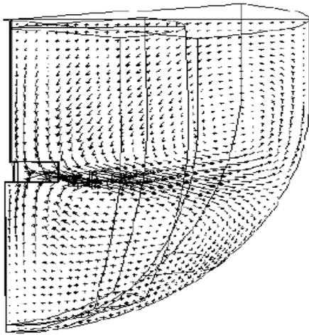
Figure 16: Velocity profile for real-lead kettle.
