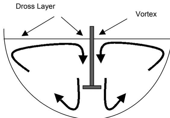
Figure 2: Kettle shape and possible flow profiles.
