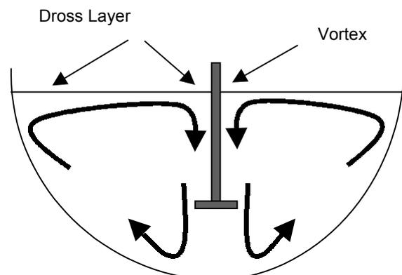
Figure 2: Kettle shape and possible flow profiles.
