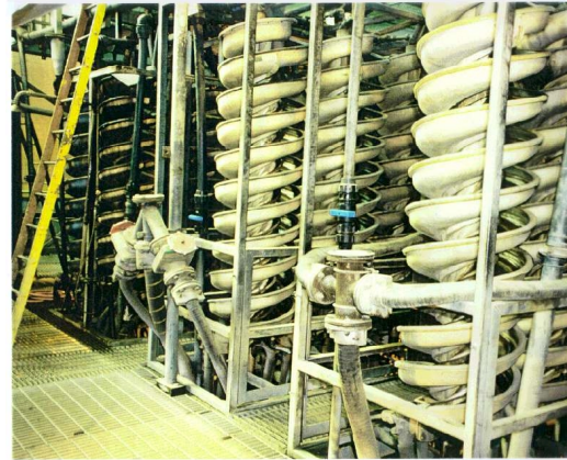
Figure 1: Spiral concentrators in the processing plant.
