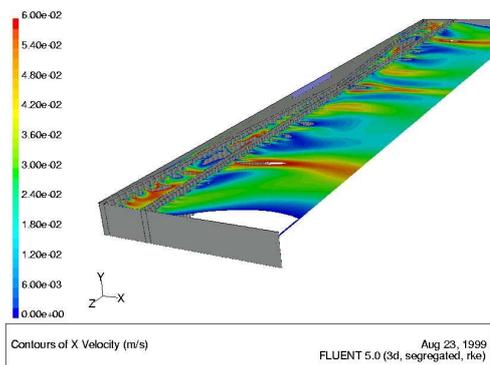
**Figure 9:** Picture showing the x velocity profile in the plane through the centre of the inlet.
