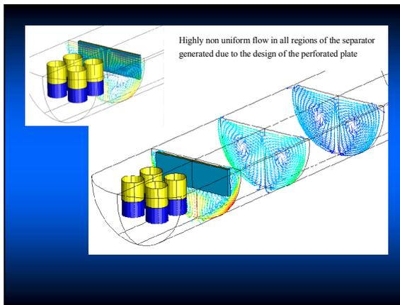
**Figure 2:** Summary of the CFD simulation of the HP Separator.
