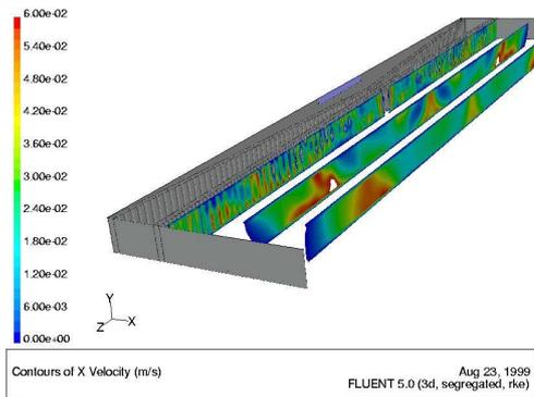
**Figure 8:** Picture showing the x velocity profile along the length of the vessel.
