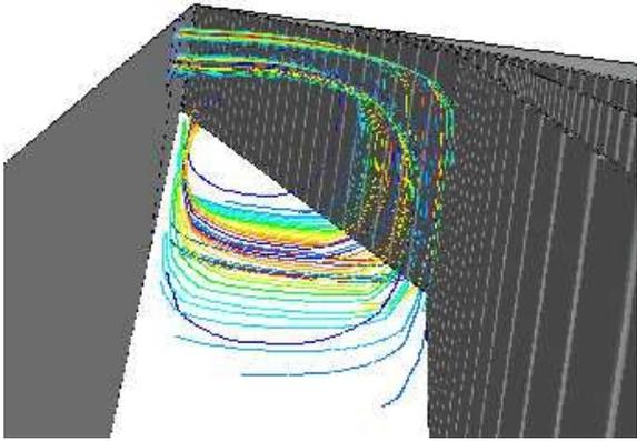
**Figure 7:** Picture showing the path lines of the fluid after it enters the vessel. A corkscrew motion is clearly seen.
