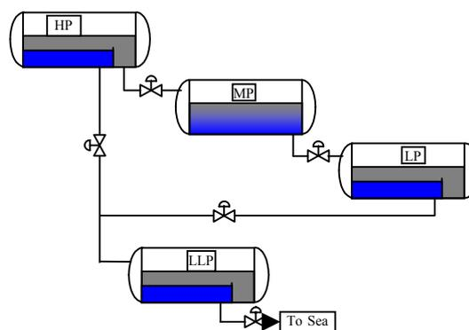
Figure 1: Typical offshore water processing scheme
