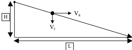
The minimum available  $V_t$  enables the calculation of the minimum droplet size that can be separated.
