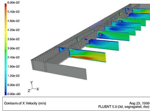
**Figure 10:** Picture showing the x velocity profile along the length of the vessel.
