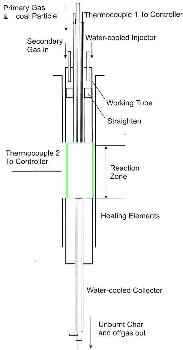
**Figure 1:** Schematic Diagram of Drop Tube Furnace
