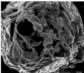
Figure 3: Particle deformation during combustion process
