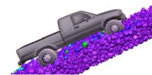
Figure 1: Simulation of vehicle driving up a 25 deg inclined slope of coarse rocks. Wheel torque (and simple tyre tread) are insufficient for vehicle to drive up the incline and significant wheel sinkage occurs for the front wheels.
